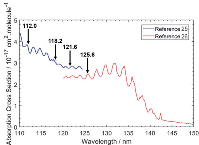
Fig. 1 VUV absorption spectrum of C<sub>2</sub>H<sub>6</sub> from ref. 25 and 26. The data from ref. 26 were extracted manually, while the data from ref. 25 were retrieved from ref. 48. The black arrows indicate the photolysis wavelengths (in nm) used in the present study.
