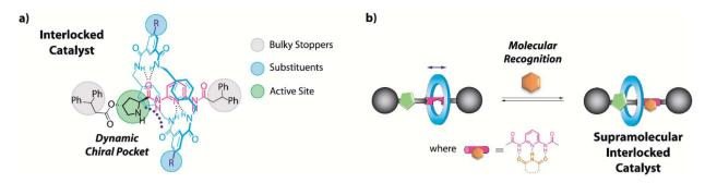
Fig. 1 Design of (a) an interlocked DAP-based organocatalyst and (b) the formation of its hydrogen-bonding supramolecular complex.
