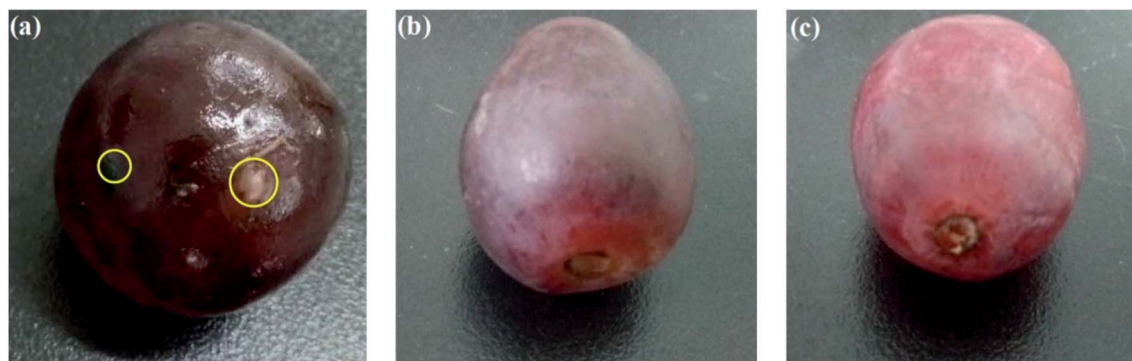
Fig. 15 Extended shelf-life of red grape packed at 37 °C for 6 days in (a) plastic wrap; (b) chitosan film; (c) chitosan-TiO 2 film. Adapted from ref. 141 with permission from Elsevier Ltd, Copyright 2017.
