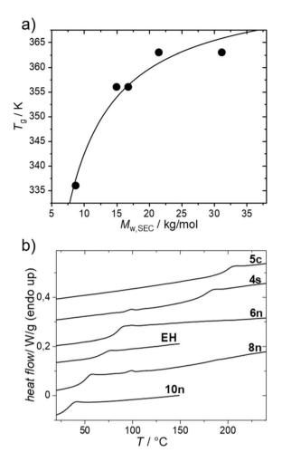
Fig. 2 Glass transition temperature of PmmpF4 from differential scanning calorimetry with 6n as a function of molecular weight (a) and for varying side chains including entry 5 (b). Conditions:  $2^{nd}$  heating, 10 K min<sup>-1</sup>, N<sub>2</sub>.
