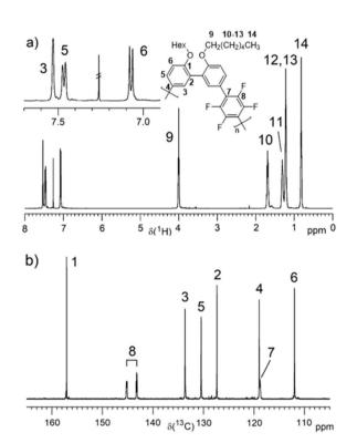
Fig. 1  $\,^{1}$ H (a) and  $^{13}$ C (b) NMR spectra of PmmpF4 (entry 2) in CDCl $_{3}$  with assignments.
