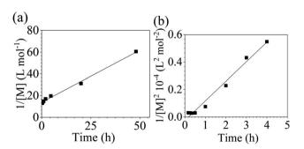
Fig. 4 Linearized kinetic plots of: (a) second-order reaction for the polycondensation of DCDPS/BPA with  $Na_2CO_3$  at 160 °C, and (b) third-order reaction for the polycondensation of DFDPS/BPA with  $Na_2CO_3$  at 140 °C.
