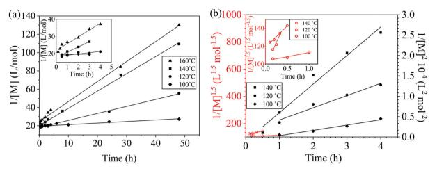
Fig. 7 Linearized kinetic plot of (a) the DCDPS/BPA reaction and (b) the DFDPS/BPA reaction at conversions <90% (hollow red markers) fit to a 2.5order rate expression (red line), and at conversions >90% (solid black markers) fit to a third-order rate expression (black line) at various temperatures with potassium carbonate as the base.
