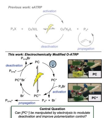
Fig. 1 Previous work demonstrated the ability to mediate ATRP using electrochemistry (top). In this work (bottom), we ask whether this principle can be applied to O-ATRP to control the concentration of PC<sup>-+</sup> and thereby control deactivation in this polymerization method. Figure inset (bottom right) demonstrates the conversion of PC to PC<sup>-+</sup> using potentiostatic bulk electrolysis.
