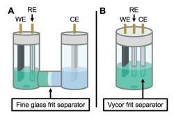
Fig. 4 Diagram of the apparatus used in this work. Originally, a modified U-cell was employed to separate the working and counter electrode compartments (A). When this separator was found to be ineffective on the time scale of eO-ATRP, a new apparatus was developed using a 5-neck electrochemical flask (see Experimental equipment in ESI†) and vycor frit separators to isolate the counter electrode (B). WE = working electrode, RE = reference electrode, and CE = counter electrode.
