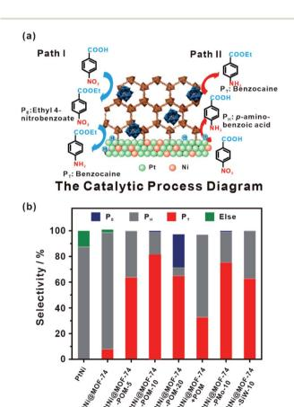
Fig. 20 (a) Schematic illustration of tandem catalytic mechanism on PtNi@MOF-74-POM. (b) Catalysis of tandem reaction with different catalysts. Reproduced with permission. Copyright 2019 The Royal Society of Chemistry.
