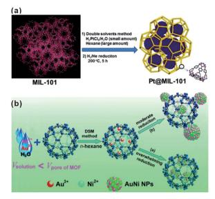
Fig. 2 (a) Schematic representation of the synthesis of Pt NPs inside the MIL-101 matrix using the double-solvent method. 48 Copyright©2012 American Chemistry Society. (b) Scheme representing the immobilization of AuNi NPs by the MIL-101 matrix using the double-solvent method combined with liquid-phase concentration-controlled reduction (CCR) strategy. 52 Copyright©2013 American Chemistry Society.
