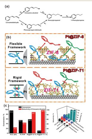
Fig. 12 (a) Reaction paths of CAL hydrogenation. (b) Schematic illustration of hydrogenation of CAL on Pt NPs embedded within flexible ZIF-8 and rigid ZIF-71, respectively. (c) Conversions and selectivity of four products of CAL hydrogenation over Pt/C-20%, Pt-PVP, Pt@ZIF-8-1%, and Pt@ZIF-71-1%. Reproduced with permission.<sup>75</sup> Copyright@2017 WILEY-VCH Verlag GmbH & Co. KGaA.
