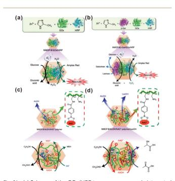
Fig. 21 (a) Scheme of the GOx/HRP two-enzyme cascade integrated in ZIF-8 NMOFs. (b) Activation of a three-enzyme biocatalytic cascade encapsulated in ZIF-8 NMOFs. (c) NAD<sup>+</sup>-mediated biocatalytic cascade of a cofactor-dependent enzyme in ZIF-8 NMOFs. (d) NAD<sup>+</sup>-mediated two-enzyme biocatalytic cascade in ZIF-8 NMOF nanoreactors. Reproduced with permission.<sup>30</sup> Copyright@2018 Nature Publishing Group.
