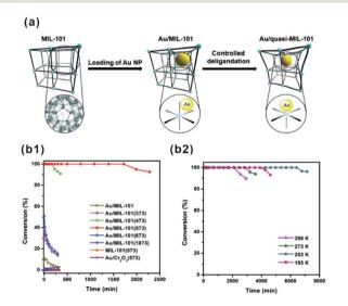
Fig. 18 (a) Schematic illustration showing the synthesis of Au/quasi-MIL-101 through controlled deligandation of Au/MIL-101. (b1) Catalytic activity in CO oxidation of different catalysts. (b2) CO oxidation at various temperatures catalyzed by Au/MIL-101(573). Reproduced with permission.<sup>178</sup> Copyright©2018 Elsevier Inc.
