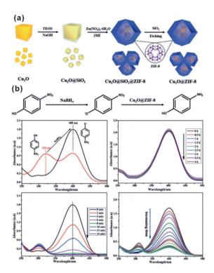
Fig. 8 (a) Schematic illustration of synthesis of the Cu<sub>2</sub>O@ZIF-8 composite, and (b) catalytic reduction equation of 4-nitrophenol to 4aminophenol using Cu<sub>2</sub>O@ZIF-8. Reproduced with permission.86 Copyright@2018 WILEY-VCH Verlag GmbH & Co. KGaA.
