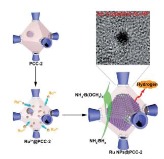
Fig. 3 Scheme representing the synthesis of fcc Ru NPs *via* PCC-2 as the template. Reproduced with permission.<sup>57</sup> Copyright@2018 Elsevier Inc.
