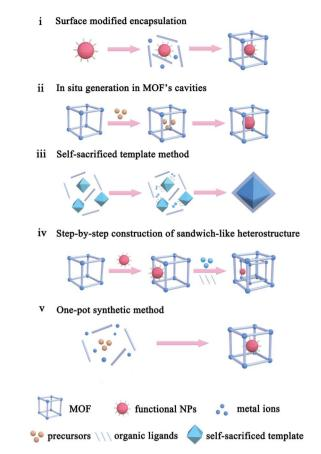
**Scheme 1** Main approaches used for the construction of MOF-based composites.
