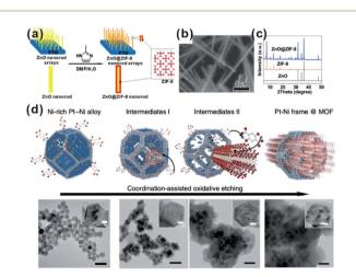
Fig. 4 (a) Scheme of ZnO@ZIF-8 nanorods synthesized by the selftemplate strategy. (b) SEM image and (c) XRD pattern of ZnO@ZIF-8 nanorods. Reproduced with permission.<sup>26</sup> Copyright@2013 American Chemistry Society. (d) Scheme and corresponding TEM images of the coordination-assisted oxidative etching process (scale bars represent 50 nm). Insets are magnified TEM images (scale bars represent 5 nm). Reproduced with permission.<sup>62</sup> Copyright@2015 Nature Publishing Group.
