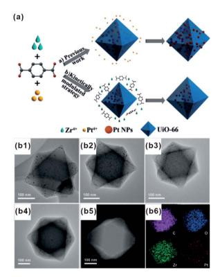
Fig. 7 (a) Incorporation of Pt NPs in MOFs through an *in situ* one-step strategy and a kinetically modulated *in situ* one-step strategy. (b1–b4) TEM images of Pt@UiO-66 nanocomposites prepared by different volume ratios of  $H_2/air$ . A (b5 and b6) HAADF-STEM image and corresponding elemental mapping of Pt@UiO-66. Reproduced with permission.<sup>77</sup> Copyright©2016 WILEY-VCH Verlag GmbH & Co. KGaA.
