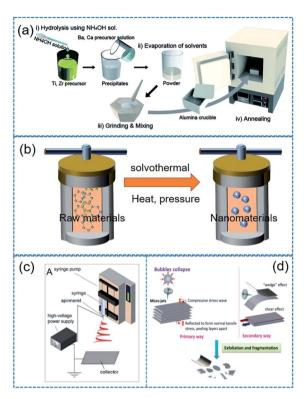
Fig. 4 Illustrated flow chart of (a) sol-gel, (b) solvothermal/hydrothermal, (c) electrospinning, (d) mechanical exfoliating process. This figure has been adapted/reproduced from ref. 144, 156 and 159 with permission from American Chemical Society, copyright 2017; Royal Chemical Society, copyright 2015; and Royal Chemical Society, copyright 2016, respectively.
