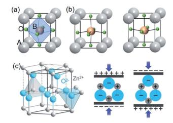
Fig. 1 Stereoscopic illustration of ABO<sub>3</sub> perovskite structures (a) with centrosymmetry and (b) with non-centrosymmetry by B ions upwards or downwards. (c) Schematics of wurtzite structure (ZnO as an example) and the related piezoelectric effect. This figure has been adapted/reproduced from ref. 53 with permission from John Wiley & Sons, copyright 2016.
