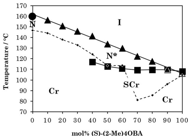
Fig. 2 Phase diagram of binary mixtures of 4OBA and (S)-(2-Me)4OBA, where  $\blacklozenge$  represents the melting point,  $\bullet$   $T_{NI}$ ,  $\blacktriangle$   $T_{N^*}$ , and  $\blacksquare$   $T_{SCrNI}$ . An unfilled triangle represents a virtual transition temperature.
