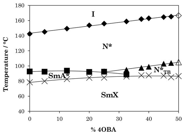
Fig. 4 Dependence of phase behaviour of the 1OB6OS:4OBA:(S)-(2-Me)4OBA series of ternary mixtures on the molar percentage of achiral H-bond donor 4OBA, where  $\blacklozenge$  represents  $T_{N^*}$ ,  $\blacksquare$   $T_{SmA^*}$ ,  $\blacktriangle$   $T_{N^*_{TB}N^*}$  and  $\times$   $T_{N^*_{TB}/SmA-SmX}$ . Unfilled diamond and triangle represent conventional  $N-I$  and  $N^*_{TB}-N^*$ , respectively. Melting points omitted for clarity.
