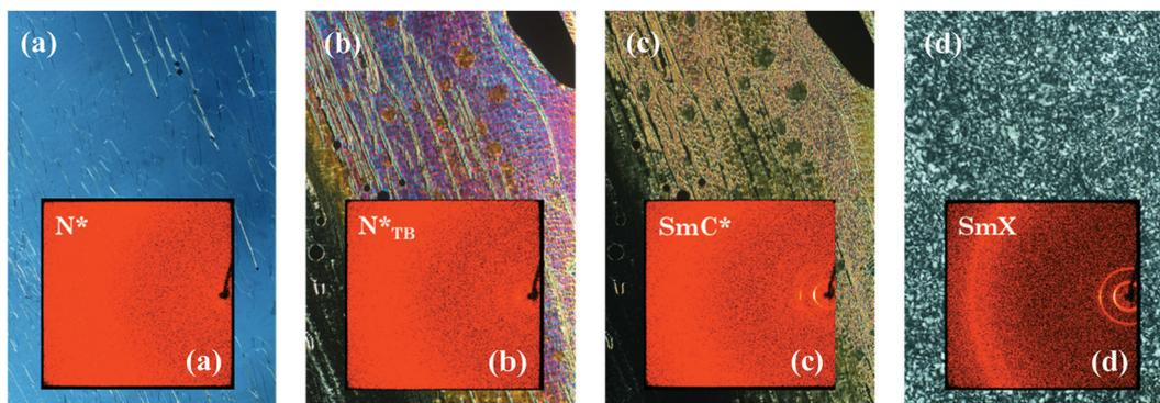
**Fig. 7** POM images and associated X-ray diffraction patterns (insets) for CB6OBA:(S)-(2-Me)4OS in the (a) N\*, (b) N\*<sub>TB</sub>, (c) SmC\* and (d) SmX phases.
