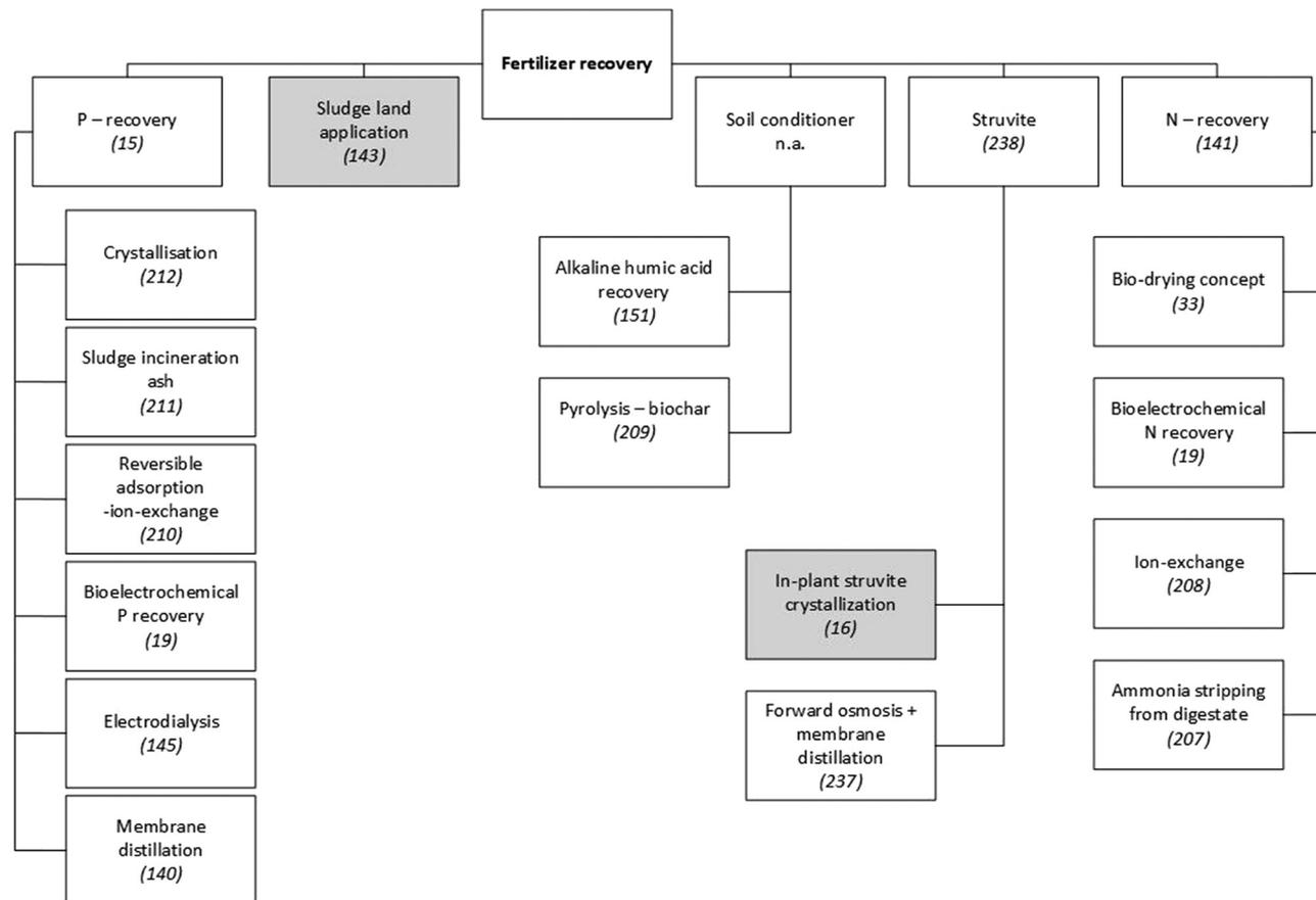
**Fig. 3** Examples of technologies to recover fertiliser from municipal WWTPs. Since a detailed presentation and discussion of these technologies is beyond the scope of this paper, scientific publications that explain or review them are referenced. Grey shading indicates techniques that have been applied on a large scale in municipal WWTPs. Unshaded boxes show technologies that are not widely applied.<sup>15,16,19,33,140,141,143,145,151,207–212,237,238</sup>
