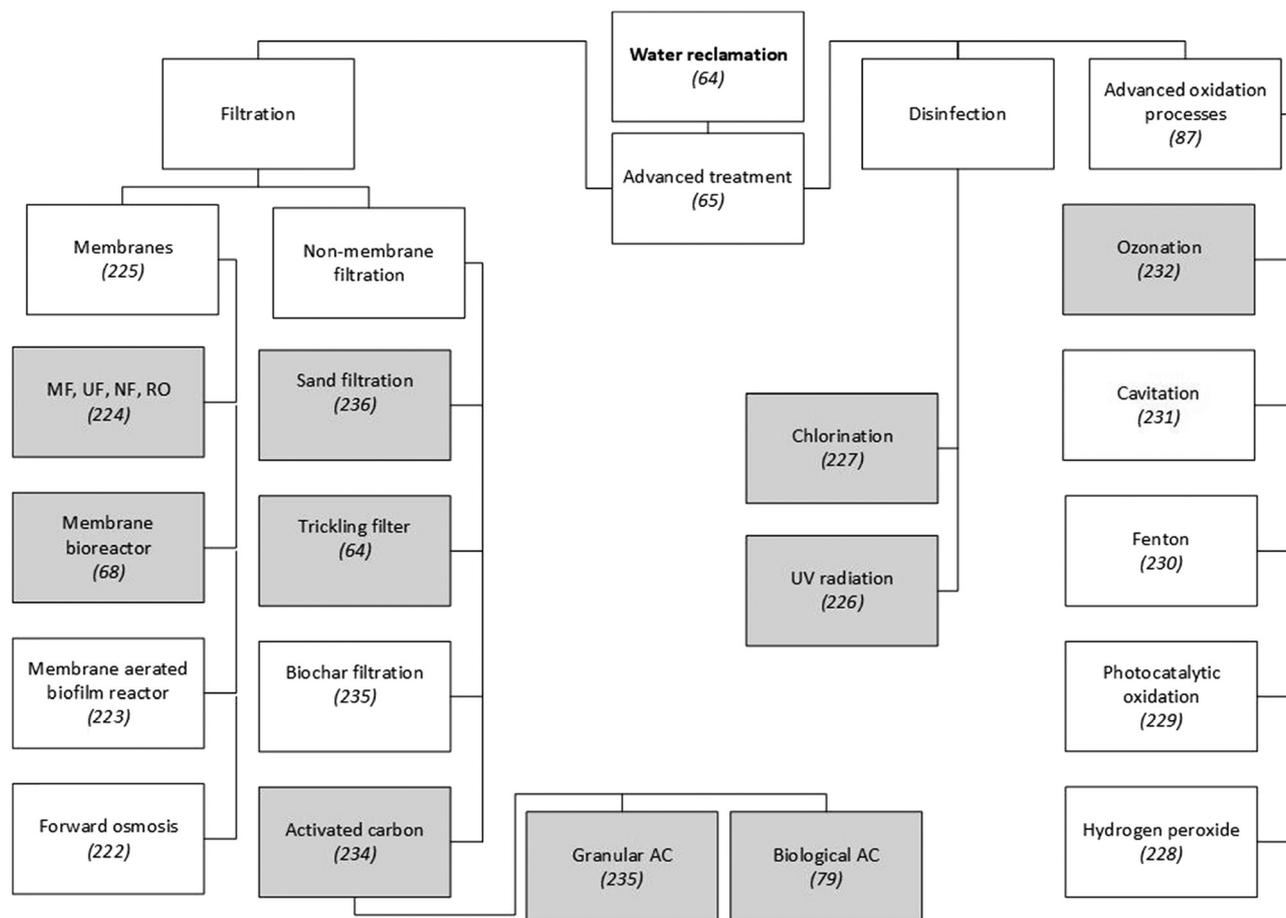
**Fig. 1** Examples of technologies to reclaim water from municipal WWTPs. Since a detailed presentation and discussion of these technologies is beyond the scope of this paper, scientific publications that explain or review them are referenced. Grey shading indicates techniques that have been applied on a large scale in municipal WWTPs. Unshaded boxes show technologies that are not widely applied.<sup>64,65,68,79,87,222–232,234–236</sup>
