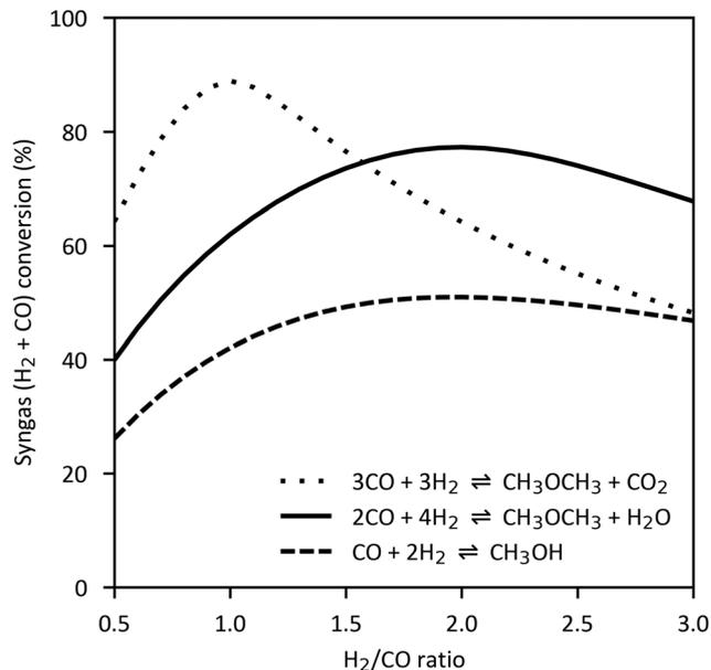
Fig. 12 Syngas conversion for methanol synthesis and DME synthesis reactions as function of H<sub>2</sub>/CO ratio (260 °C, 50 bar, own illustration of ref. 30 based on Aspen Plus Simulation).
