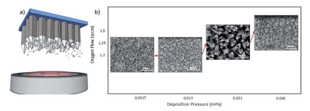
Fig. 1 (a) Schematic view of the  $Co_3O_4$  NRs synthesis *via* physical vapor deposition. (b) The morphological changes of the deposited  $Co_3O_4$  films with respect to their deposition pressure onset on FTO substrate.
