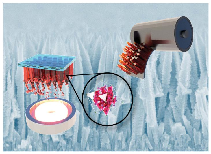
Showcasing a study on a new synthesis of  $\mathrm{Co_3O_4}$  tapered nanorods through plasma assisted vapor solid deposition, for application in energy conversion and storage, by a group of researchers led by Prof. Alberto Vomiero from Luleå University of Technology.
