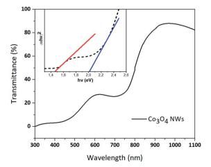
Fig. 4 Transmittance spectra of the  $Co_3O_4$  NRs grown on glass substrate, 400 nm long. (Inset) Band gap measurement of  $Co_3O_4$  nanorods using Tauc plot method.
