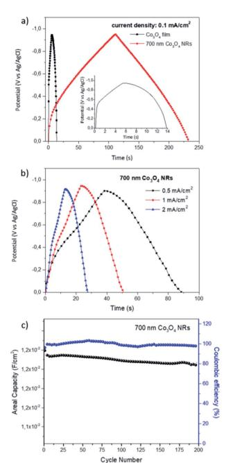
Fig. 7 (a) Charge-discharge profile of 700 nm  ${\rm Co_3O_4}$  NRs and a PVD deposited film (nominal thickness 400 nm). (b) Charge-discharge behavior of 700 nm electrode under different current densities. (c) Cyclic performance for 200 cycles at 0.1 mA cm $^{-2}$ .
