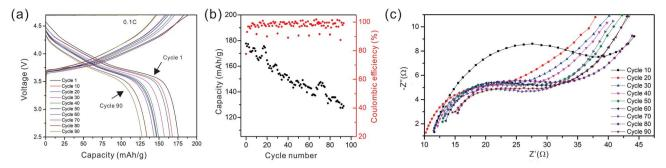
(a) The cycling curves, (b) capacity and coulombic efficiency, and (c) impedance curves of the hybrid cell from the 1st to the 90th cycle.
