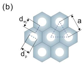
Fig. 8 (a) The 3D model and (b) top view of the simplified honeycomb structure of the porous LLZO scaffold.
