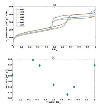
Fig. 4 (a)  $N_2$  adsorption isotherms of the mixed MO photocatalysts (b) impact of increasing fraction of  $TiO_2$  on BET specific surface area.
