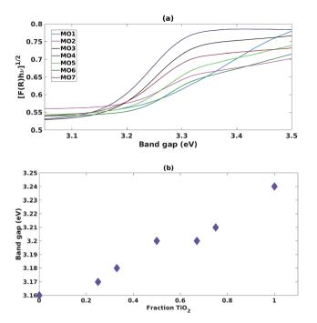
Fig. 2 (a) Tauc plots for mixed MO photocatalysts (b) impact of increasing fraction of  $TiO_2$  on band gap.
