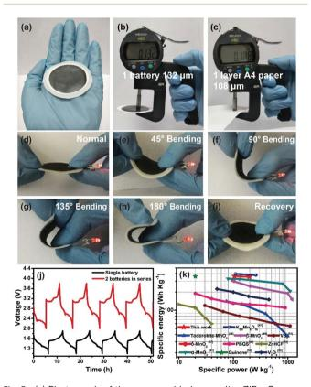
Fig. 5 (a) Photograph of the as-assembled paper-like ZIBs. Comparison between the thickness of (b) the membrane-like ZIBs and (c) standard A4 printing paper. (d–i) The flexible membrane-battery powers a red LED indicator at various bending angles. (j) Galvanostatic charge/discharge curves of a single battery and two batteries connected in series at 0.05A  $\rm g^{-1}$ . (k) Ragone plot related to energy and power densities of recently reported ZIBs and the present work.
