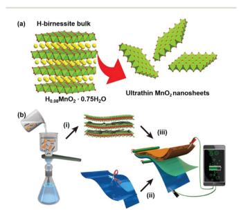
Fig. 1 (a) Crystal structure evolution by liquid exfoliation of the Hbirnessite bulk into single-atomic layers. (b) Schematic illustration of (i) the vacuum-assisted filtration strategy to fabricate the freestanding MnO<sub>2</sub>/MWCNT hybrid membrane; (ii) trimmed zinc foil as the anode material; (iii) assembly of a proof-of-concept paper-like ZIB.
