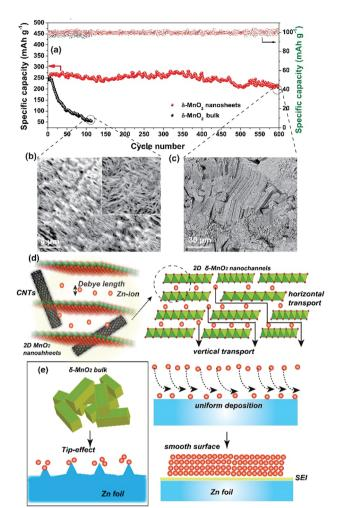
Fig. 4 (a) Cycle performance and coulombic efficiency of the MnO<sub>2</sub>-based ZIBs in a voltage range of 1.0–1.9 V at 0.1 A g<sup>-1</sup>. SEM images of the Zn foil anode surface morphology in the (b)  $\delta$ -MnO<sub>2</sub> bulk and (c) flexible MnO<sub>2</sub>/MWCNT ZIBs after 600 cycles. Schematic illustration of the Zn<sup>2+</sup> transport process in (d) 2D nanofluidic channels and (e) the  $\delta$ -MnO<sub>2</sub> bulk, respectively.
