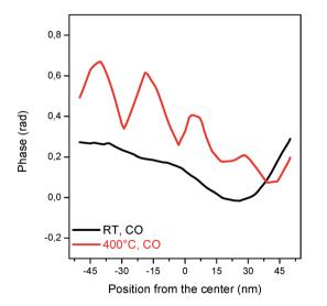
Fig. 4 Line scans of the phase at RT (black) and 400  $^{\circ}$ C (red) under CO/O<sub>2</sub>. The line scan corresponds to the values of the position of the dashed line shown (for 400  $^{\circ}$ C) in Fig. 2a.
