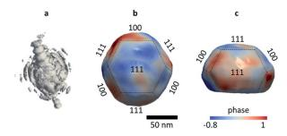
Fig. 1 (a) 3D diffraction pattern obtained by rocking scans around the (111) Bragg peak of a 120 nm Au/TiO2 nanoparticle in air at RT. The corresponding 3D reconstruction with a 30% isosurface seen from (b) top and (c) side views scaled with the phase. The facet orientations are shown.
