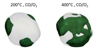
Fig. 3 Distribution of the maximum phase shift [0.4–1.1 rad] of the same Au/TiO $_2$  nanoparticle under CO/O $_2$  at 200 °C and 400 °C from the bottom view. The crystal at 200 °C shows highly distorted areas concentrated at the surface of three edges. At 400 °C, a complex network is present with highly distorted areas crossing the entire volume of the crystal and connecting the three regions highlighted at 200 °C.
