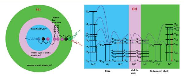
Fig. 5 (a) Schematic illustration of the non-radiative ET mechanism of  $Tm^{3+} \leftarrow Yb^{3+} \leftarrow Nd^{3+} \rightarrow Yb^{3+} \rightarrow Fr^{3+}$  in CSS (5 mol%  $Er^{3+}$ ) UCNPs (808 nm laser excitation). (b) Schematic illustration of ET pathways to produce bright UCL from both the core (blue,  $Tm^{3+}$ ) and the outermost shell (red and green,  $Er^{3+}$ ) in the same CSS UCNPs upon 808 nm excitation.
