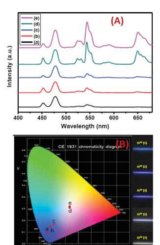
Fig. 9 (A) UCL spectra (B) corresponding 'Commission Internationale de l'Eclairage' (CIE) and digital images of CSS UCNPs. a, b, c, d and e in the CIE diagram indicate the corresponding UCNPs, having Er3+ concentrations 1, 2, 3, 5 and 7 mol%, respectively, in the outermost shell. Digital images are taken using an 808 nm laser, 10 W cm<sup>-2</sup> (without using any filter).
