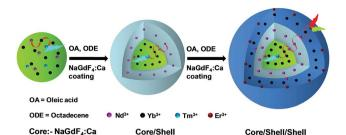
**Scheme 1** Schematic illustration of the synthesis of CSS UCNPs following a seed-mediated layer-by-layer growth method.
