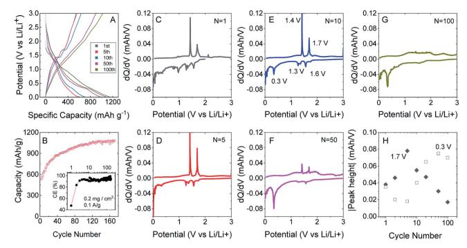
Fig. 4 Performance of composites of MoO<sub>2</sub> flakes/SWCNTs (20 wt%) as lithium ion battery anodes. (A) Galvanostatic charge-discharge curves for different number of cycles. (B) Cycling (charging) capacity versus cycle number at  $0.1 \, \text{A g}^{-1}$  with coulombic efficiency shown in the inset. (C-G) Differential curves associated with voltage profiles for different cycle numbers. (H) Absolute heights for the peaks at 1.7 V (insertion) and 0.33 V
