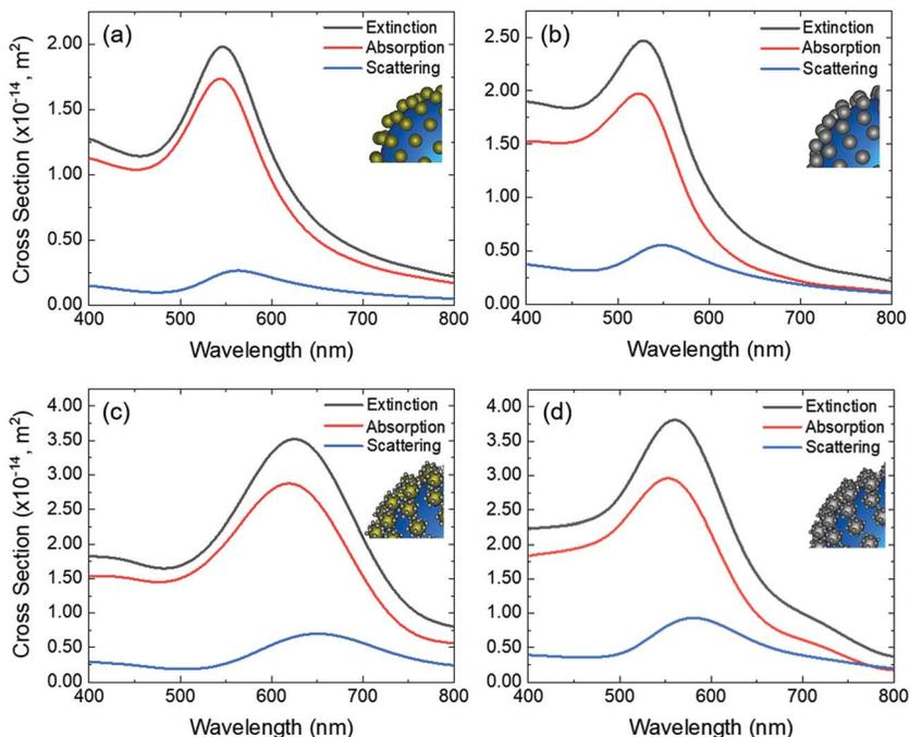
Fig. 2 Numerical simulations of extinction, absorption and scattering cross sections for (a) 15 nm diameter Au nanoparticles on  $\text{SiO}_2$  and (b–d)  $\text{SiO}_2$ –Au–Pt heterostructures with (b) a 0.5 nm thickness of Pt shell, (c) a 2 nm radius of Pt seeds and (d) a 0.5 nm Pt shell and 2 nm radius Pt seeds. Au nanoparticle size is the same for all simulations.
