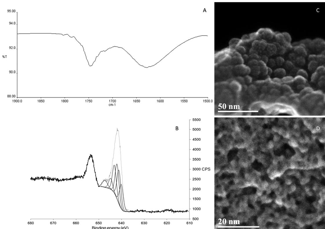
**Fig. 2** Characterization of KMH-1: (A) expansion of the metal hydride stretch region of the infrared spectrum of KMH-1 after 2nd hydrogenation; (B) manganese  $2p_{3/2}$  region of XPS of KMH-1 after 2nd hydrogenation; (C) STEM-SE image of powder morphology of KMH-1 as-synthesized at a scale of 50 nm (magnification 700 kX); (D) STEM-SE of pore structure of KMH-1 after 2nd hydrogenation at a scale of 20 nm (magnification 1.8 MX).
