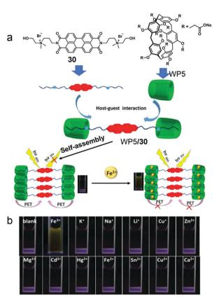
Fig. 23 (a) Chemical structures of the host and guest compounds and a cartoon representation of the Fe<sup>3+</sup> ion sensing mechanism. (b) Photographs of WP5/30 supra-amphiphile solutions after adding various metal ions under UV light. Adapted with permission from ref. 95. Copyright 2017 American Chemical Society.
