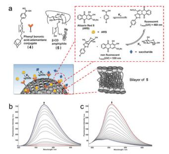
Fig. 5 (a) Schematic representation of the formation of bilayer vesicles with sensing ability. (b) Fluorescence spectra of titration of Alizarin Red S (ARS) with 4. (c) Fluorescence titration of 4 with fructose in the presence of ARS and bilayers vesicles (\(\beta\text{-CDV}\). Adapted with permission from ref. 33. Copyright 2017 John Wiley and Sons.
