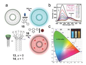
Fig. 11 (a) Schematic representation of the formation of the broadspectrum tunable photoluminescent materials. (b) Fluorescence spectra of the 14/15 assembly in PBS buffer with different concentrations of 16,  $\lambda_{\rm ex}$  = 369 nm. (c) The luminescent color changes of the **14/15** assembly with different concentrations of 16 in PBS buffer. Adapted with permission from ref. 62. Copyright 2016 John Wiley and Sons.
