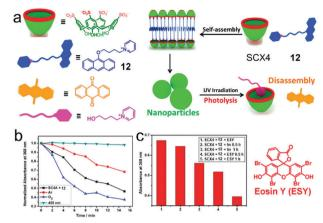
Fig. 10 (a) Schematic representation of the photolyzable supraamphiphilic system. (b) The absorbance of the SCX4/12 assembly at 368 nm upon irradiation for different amounts of time. (c) The absorbance of the SCX4/12 assembly at 368 nm in the absence and presence of eosin upon irradiation at 520 nm for different amounts of time. Adapted with permission from ref. 57. Copyright 2017 American Chemical Society.
