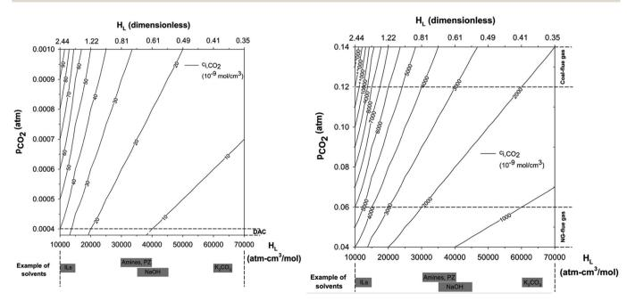
Fig. 25 Interfacial concentration of  $CO_2$ ,  $c_i$ , based upon Henry's law for DAC (left) and the flue gas of natural gas and coal (right)
