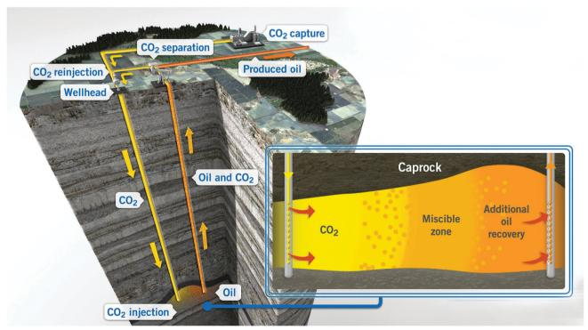
Fig. 19 Schematic diagram of CO<sub>2</sub>-EOR process. Source: Global CCS Institute. 964
