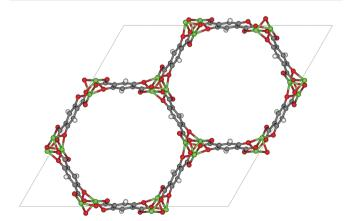
Example of a MOF. Here the structure of Mg-MOF-74 is shown. This MOF exhibits the highest reported CO<sub>2</sub> uptake for unfunctionalised adsorbents
