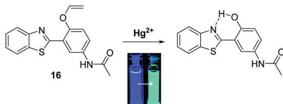
Scheme 17 Vinyl-ether protected ESIPT probe 16 , a species that proved useful for the selective detection of Hg 2+ . Measurement conditions: PBS (pH 7.4) containing 1% ACN. Adapted with permission from ( Org. Lett. , 2011, 13 , 3422–3425). Copyright (2011) American Chemical Society.
