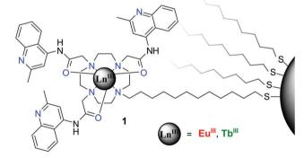
Fig. 25 The structure of AuNPs functionalised logic gate mimics, with two types of quinoline—cyclen complexes (Ln = Eu( $\parallel$ ) or Tb( $\parallel$ )), functionalised to the Au–surface through thiol linkages.
