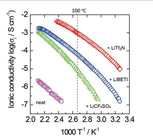
Fig. 4 Arrhenius plots of ionic conductivity for neat 1 and its lithium-salt complexes. The lithium-salt content is 50 mol% for all the complexes.
