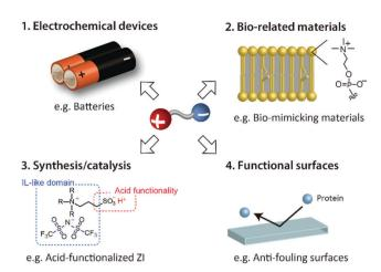
Fig. 14 Expected applications of IL-derived ZIs.
