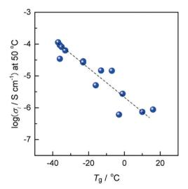
Fig. 5 The relationship between ionic conductivity at 50  $^{\circ}$ C and  $T_{\rm q}$  for ZI/lithium-salt mixtures.
