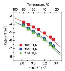
**Fig. 7** Arrhenius plots of ionic conductivity for ZI/lithium-salt complexes. The lithium-salt content is 50 mol% for all the complexes.
