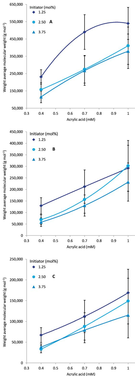
**Fig. 6** Molecular weight increases for higher monomer feed. Lower temperature will increase the molecular weight. Residence time is 30 minutes, A: polymerisation at 70 °C, B: polymerisation at 80 °C and C: polymerisation at 90 °C.
