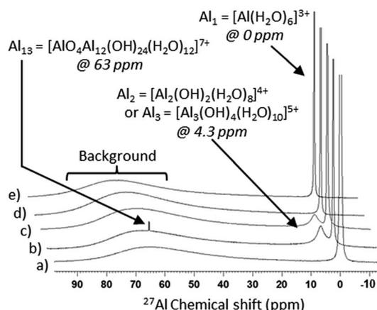
Fig. 1  $^{27}\text{Al}$  NMR spectra for (a) aqueous solution of  $\text{Al}(\text{NO}_3)_3 \cdot 9\text{H}_2\text{O}$ ,  $[\text{Al}] = 1.6 \text{ M}$  (b) solution of  $\text{Al}(\text{NO}_3)_3 \cdot 9\text{H}_2\text{O}$  in an aqueous NaOH solution with a NaOH : Al molar ratio of 0.77 : 1 and (c–e) remnant solution after hydrothermal treatment of precursors with initial NaOH : Al molar ratio of 0.77 : 1 after 20 hour at (c) 150 °C (d) 180 °C and (e) 200 °C.
