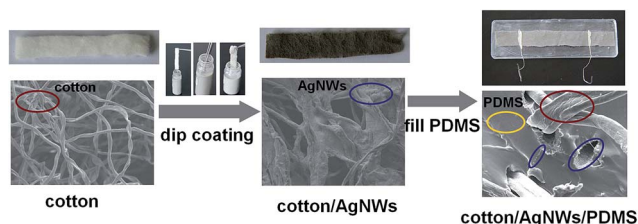
Fig. 1 Schematic diagram of the fabrication procedure of cotton–AgNWs–PDMS stretchable conductor.
