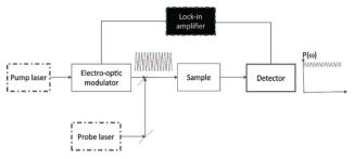
Fig. 1 Schematic for CW or pulsed SRS showing a modulated pump beam and an unmodulated probe beam. Following interaction with the sample, lock-in techniques can be used to detect the SRL in the pump beam or SRG in the probe beam by removing the unwanted one using a bandpass filter (SRL) or a long pass filter (SRG).
