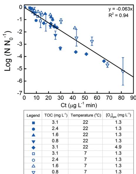
Fig. 1 Summary of *L. pneumophila* inactivation at 7 and 22 °C with various initial TOC loadings and initial ozone concentrations generated when the ozone generator was driven at 50 V ( $C_{gi} = 1.3 \text{ g m}^{-3}$ ) and 120 V ( $C_{gi} = 4.9 \text{ g m}^{-3}$ ). Data plotted are average values and standard deviations of at least three replicates.
