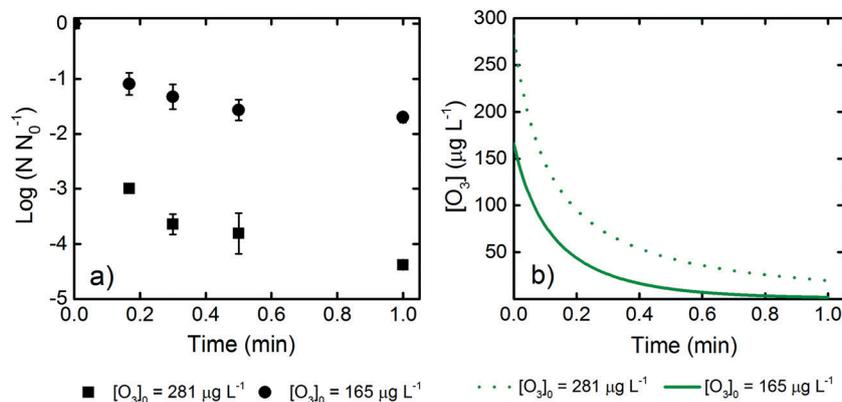
**Fig. 7** At 22 °C (a) the effect of HRT on *L. pneumophila* inactivation, at two initial ozone concentrations and a WOM loading of 3.1 mg C L<sup>-1</sup> in a semi-batch reactor; (b) the profile of two initial dissolved ozone concentrations as a function of HRT. The data plotted in (a) are average values and standard deviations of three replicates. The dashed and solid curves in (b) are the results of calculations.
