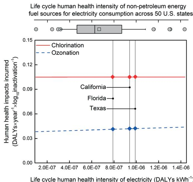
**Fig. 4** The relationship between the incurred human health impacts and the life cycle human health intensity (in the unit of DALYs kW h<sup>-1</sup>) of non-petroleum energy fuel sources for the consumed electricity across 50 U.S. states. Three states with the heaviest reliance on reclaimed water, California, Florida, and Texas, are marked.
