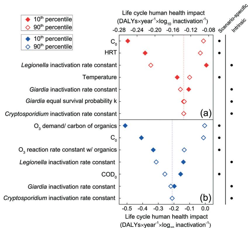
Fig. 5 The top seven input parameters to which human health impacts are most sensitive, for chlorination (a) and microplasma ozonation (b), expressed in DALYs × year<sup>-1</sup> × log<sub>10</sub> pathogen inactivated<sup>-1</sup>. Sensitivity analysis for the rest of the parameters can be found in Fig. S4a and b in the ESI.†
