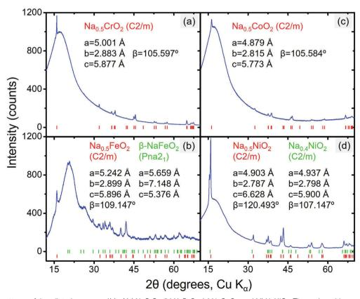
Fig. 5 Diffraction patterns of desodiated compound(s) of (a) NaCrO<sub>2</sub>, (b) NaFeO<sub>2</sub>, (c) NaCoO<sub>2</sub>, and (d) NaNiO<sub>2</sub>. The peak positions and refined structure data are also displayed; the hump at  $\sim 15^{\circ}$  in all four figures originates from the Kapton sample holder (the diffraction pattern of the empty sample holder is presented in Fig. S3, ESI†)
