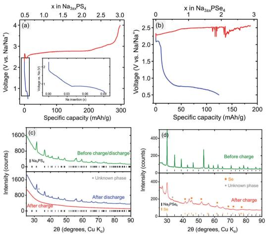
Fig. 3 Electrochemical cycling of the  $Na_3PX_4$  (mixed with carbon) cathode composite at constant current (2.604 mA  $g^{-1}$  for  $Na_3PS_4$  and 2.404 mA  $g^{-1}$  for  $Na_3PS_4$ , showing the stability window of (a)  $Na_3PS_4$  and (b)  $Na_3PS_4$ . Diffraction patterns of the (c)  $Na_3PS_4$  cathode composite before and after being fully charged/discharged and (d)  $Na_3PS_4$  cathode composite before and after being fully charged.
