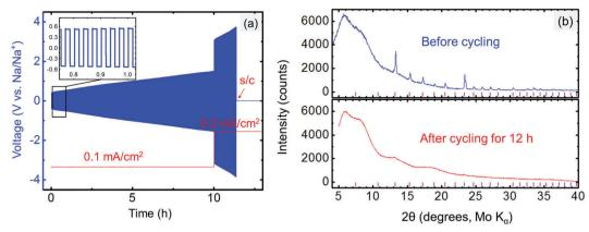
Fig. 8 (a) Electrochemical cycle for Na|Na<sub>3</sub>PSe<sub>4</sub>|Na symmetric cell; a short circuit (s/c) occurred after cycling for 11.4 h. (b) XRD results for Na<sub>3</sub>PSe<sub>4</sub> before and after cycling for 12 h (1 min per cycle); the tick marks indicate Na<sub>3</sub>PSe<sub>4</sub> peaks.
