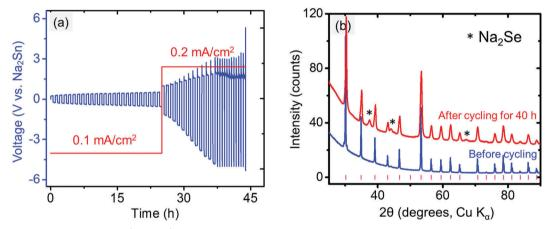
Fig. 9 (a) Electrochemical cycling of Na<sub>2</sub>Sn|Na<sub>3</sub>PSe<sub>4</sub>|Na<sub>2</sub>Sn symmetric cell. (b) XRD patterns of Na<sub>3</sub>PSe<sub>4</sub> before and after cycling for 40 h (60 min per cycle); the tick marks indicate Na<sub>3</sub>PSe<sub>4</sub> peaks.
