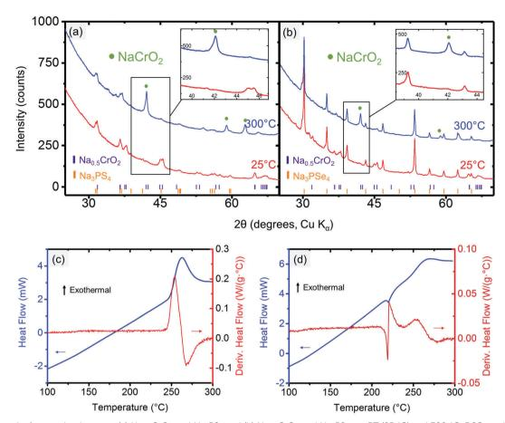
Fig. 6 XRD results for reaction between (a)  $Na_{0.5}CrO_2$  and  $Na_3PS_4$  and (b)  $Na_{0.5}CrO_2$  and  $Na_3PSe_4$  at RT (25 °C) and 300 °C. DSC results for reaction between (c)  $Na_{0.5}CrO_2$  and  $Na_3PS_4$  and (d)  $Na_{0.5}CrO_2$  and  $Na_3PSe_4$ .
