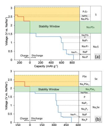
Fig. 2 Calculated stability window and decomposition products for (a) Na<sub>3</sub>PS<sub>4</sub> and (b) Na<sub>3</sub>PSe<sub>4</sub>. The green shaded region is the thermodynamically stable voltage window, and the yellow shaded region is the additional voltage range that could be kinetically stabilized.
