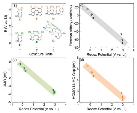
Fig. 1 (a) The calculated redox potentials of 5,6-dihydroxyindole and 5,6-indoleguinone monomers and their oligomers (dimers and trimers). The correlations of the redox potentials of the molecules in (a) with their electronic properties, namely (b) EA, (c) LUMO, and (d) HOMO-LUMO gap.
