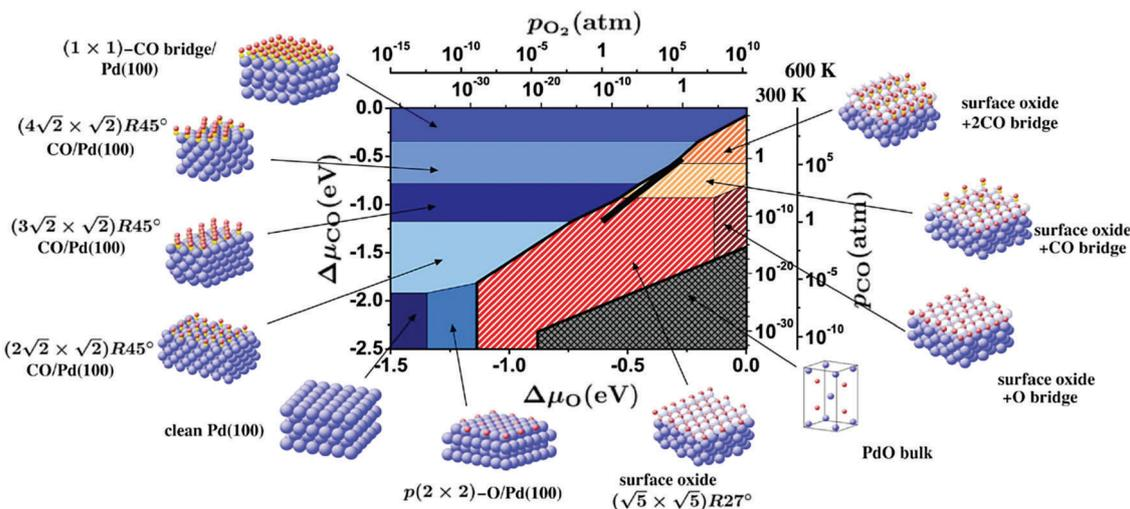
Fig. 20 Surface phase diagram of the Pd(100) surface in equilibrium with the gas phase (with the restriction that CO cannot react with O<sub>2</sub>). The black bar indicates relevant reaction conditions (101 kPa, 300–600 K). Ball models visualize the different structures (metallic Pd, blue; oxidized Pd, gray/light blue; O, red; C, yellow). Reproduced from ref. 130 with permission from the American Physical Society, copyright 2007.
