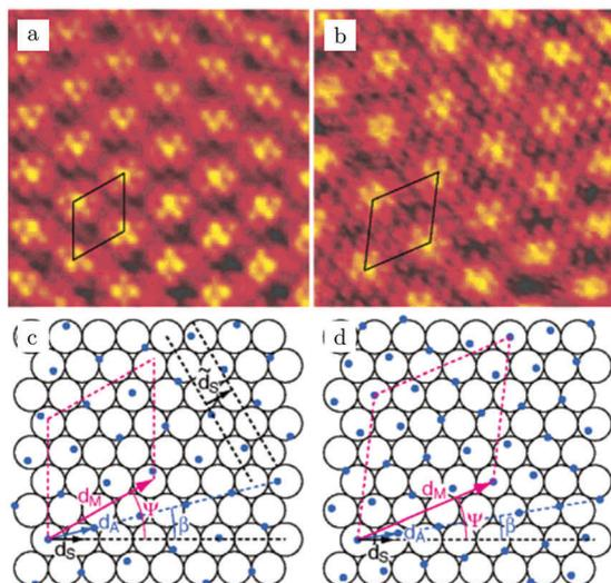
Fig. 4 STM images, RT,  $5.5 \times 5.5 \text{ nm}^2$  [(a)  $10^{-2}$  hPa CO and (b) 958 hPa CO] and ball models (c and d) of two examples of moiré patterns induced by CO overlayers on Pt(111). (d) is a model of the saturation structure of CO(ads)/Pt(111), the  $(\sqrt{19} \times \sqrt{19})R23.4^\circ$ -13 CO structure. Reproduced from ref. 53 with permission from the American Chemical Society, copyright 2004.
