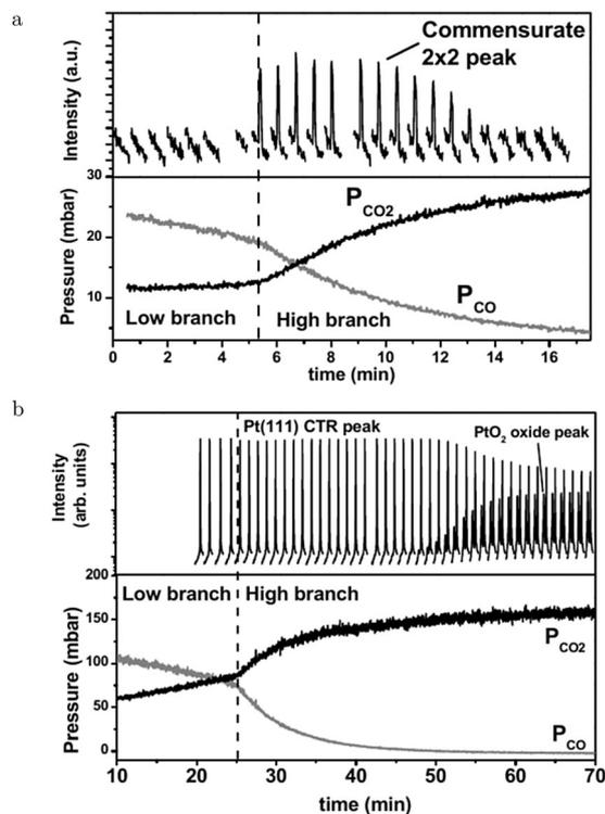
Fig. 6 Two sets of measurements in 480–500 hPa O<sub>2</sub> after a 130–150 hPa CO pulse at 570 (a) and 495 K (b). Bottom panels present the QMS data. As CO was depleted the reactivity switched to the higher activity regime. Simultaneously, the surface roughened (decrease in Pt(111) CTR) and a commensurate (2 × 2) structure developed. Later in time, PtO<sub>2</sub> appeared. Reproduced from ref. 67 with permission from the author, copyright 2007.
