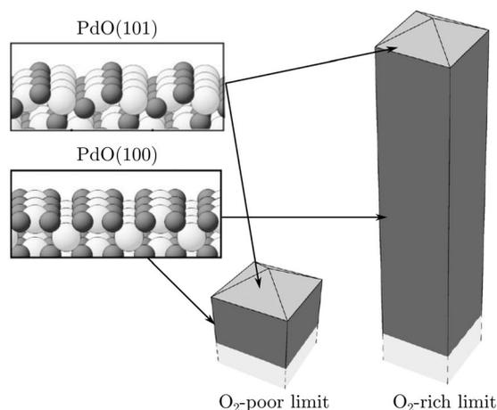
Fig. 19 Wulff construction under O<sub>2</sub>-poor (left) and O<sub>2</sub>-rich (right) conditions, based on the surface free energies derived from DFT. Insets show the only two surfaces, (100) and (101), constituting the Wulff construction. The size of the constructions is such that the (101) surface area is constant in both cases. Reproduced from ref. 136 with permission from the American Physical Society, copyright 2004.
