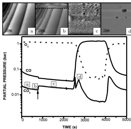
Fig. 5 STM images recorded (from bottom to top) at various stages of the experiment, in which the CO and O<sub>2</sub> partial pressures were varied at  $423\text{ K}$  at a pressure of  $125\text{ hPa}$ : (a) reduced metallic surface; (b) during the switch to higher activity; (c) oxidized surface; (d) reduced surface after increasing CO flow. The lower panel presents the QMS data. Reproduced from ref. 54 with permission from the author, copyright 2006.
