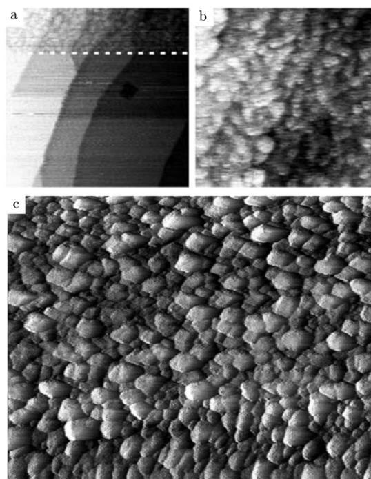
**Fig. 15** STM images (~125 kPa, 408–433 K, O<sub>2</sub>-rich mixtures) recorded (a) during the transition from a reduced to an oxidized surface; (b) slightly after; and (c) ~1 h after the transition. Reproduced from ref. 114 with permission from Elsevier, copyright 2004.
