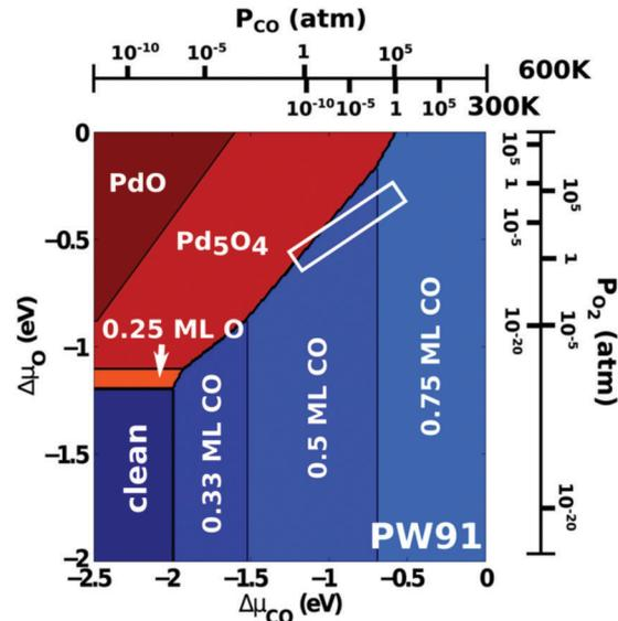
Fig. 22 Phase diagram of the Pd(111) surface in equilibrium with CO and  $O_2$  derived from DFT calculations with thermodynamic corrections. Typical reaction conditions are indicated by the white box. Reproduced from ref. 144 with permission from the American Chemical Society, copyright 2014.
