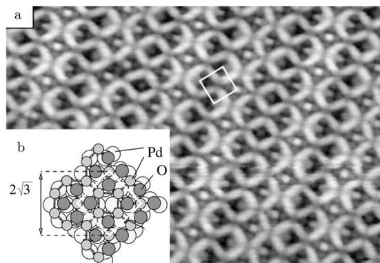
**Fig. 21** (a) STM image (10 nm wide) of  $\text{Pd}_5\text{O}_4$  on Pd(111), UHV conditions. (b) Ball model of the surface oxide, based on SXRD and DFT. Reproduced from ref. 142 with permission from the American Physical Society, copyright 2002.
