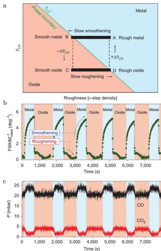
**Fig. 16** (a) Model of the spontaneous reaction oscillations on Pd(100) cycling through the surface phase diagram, plotted as a function of  $p_{\text{CO}}$  and roughness. Evolution in time (b) of the FWHM of a metallic diffraction peak (blue-colored regions) and that of the oxide (salmon-colored regions). QMS signals of CO and CO<sub>2</sub> (c) as a function of time. Reproduced from ref. 113 with permission from the Nature Publishing Group, copyright 2010.
