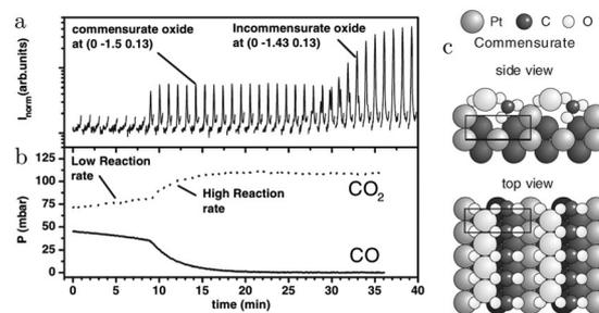
Fig. 8 SXR measurements (a) on Pt(110) in an O<sub>2</sub>-rich mixture at 625 K plotted with the QMS data (b). After 9 minutes, the reactivity increased and concurrently the commensurate oxide was observed. The DFT-based model of this oxide is plotted in (c). After a time lag, the incommensurate PtO<sub>2</sub> was also detected. Reproduced from ref. 27 with permission from the American Physical Society, copyright 2005.
