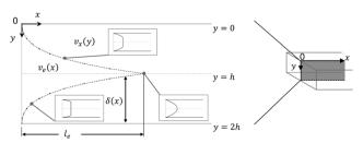
Fig. 4 Entrance region of the SPR flow cell in terms of the velocity profile.  $\delta(x)$  is the thickness of the velocity boundary layer.  $v_x(y)$ , eqn (4), is the velocity of the fluid in the velocity boundary-layer region and  $v_e(x)$ , eqn (1) and (2), is the velocity of the fluid in the potential flow region between two velocity boundary layers. Velocity profiles at three different positions are depicted.  $l_e$ , eqn (5), is the length of the entrance region.
