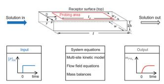
Fig. 2 Sketch of the fluid domain (upper part) and illustration of the system behavior (bottom part). The geometrical parameters are l = 2 mm, w = 0.5 mm, h = 0.01 mm,  $l_p = 1.8$  mm, and  $w_p = 0.2$  mm. [P]<sub>in</sub> is the inlet concentration of the bionanoparticle solution.  $m_{PR_n}(t)$  is the amount of adsorbed bionanoparticles at the receptor surface.
