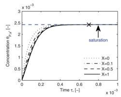
Fig. 11 Dynamic evolution of local virus concentration at the receptor surface.  $\theta_{P,s}$  is simulated by eqn (23) at different locations, X in the flow channel. The parameters used in the simulation are the same as in Fig. 10, except an increase in time to 110 minutes. The cross shows the approximate starting point of the saturation period and the saturation value is marked by the blue line.
