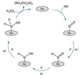
Scheme 1 Proposed mechanism for the reduction of NO to NH2OH over isolated Fe sites.
