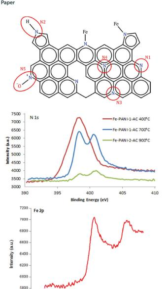
**Fig. 4** Top: Representation of a graphitic carbon material with the different possible N configurations. Middle: N 1s XPS signal as a function of the pyrolysis temperature used in the synthesis of Fe-PANI-AC. Bottom: Fe 2p XPS signal of Fe-PANI-AC-1.
