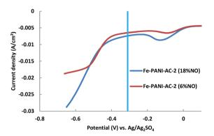
Fig. 5 Top: LSV plots of the electrocatalysts under study with 6% NO in N<sub>2</sub> as a cathode feed. Bottom: LSV plots of Fe-PANI-AC-2 with 6 and 18% NO in the feed. The part of the plot at more negative potential relative to the standard potential for the reduction of NO to NH<sub>2</sub>OH (marked by the vertical line at  $-0.31~V~vs.~Ag/Ag_2SO_4)$  is the region of interest for this study.
