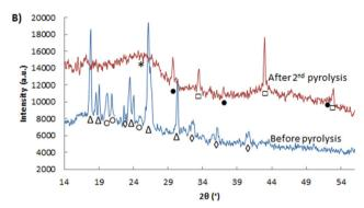
Fig. 1 X-ray diffractograms of: (A) Fe-PANI-AC-1 and (B) Fe-PANI-AC-2. The peaks in the XRD pattern are identified as follows:  $\triangle$  is  $(NH_4)_2S_2O_8$ .  $\Diamond$  is  $NH_4CI$ ,  $\bigcirc$  is polyaniline,  $\square$  is FeS,  $\blacksquare$  is Fe3,  $\square$  and  $\square$  is graphitic carbon.
