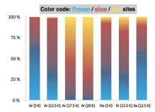
Fig. 3 Mole fractions of frozen, slow, and fast tunnelling sites in different noble gas matrices at several temperatures
