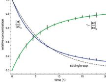
Fig. 2 Time evolution of H<sub>2</sub>CO<sub>3</sub> conformer concentrations in an Ar matrix at 20 K after NIR irradiation. Blue and green curves result from the global, nonlinear least-squares fit of the multi-exponential kinetic model to three and five IR bands of 1ct and 1cc, respectively. The dashed curve is the best single-exponential fit for 1ct.
