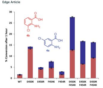
Fig. 3 The % conversion of anthranilic 4, by PrnA mutants, and ratios of products 5- and 3-chloroanthranilic acid ( $4a \div 4b$ ) after 1 hour with halogenase enzyme ( $10 \mu M$ ) and substrate (0.5 m M).
