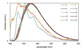
Fig. 6 Emission spectra of the complexes 4-6 and 16-22 (2 wt% in
