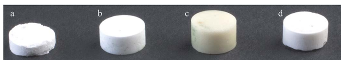
Fig. 12 Micrographs of tablets made from (a) paracetamol Form I and (b) to (d) cocrystals of paracetamol with theophylline, naphthalene and oxalic acid respectively. Tablet (a) is poorly formed as a result of the inappropriate packing of the molecules in the lattice, whereas the cocrystal structures are amenable to deformation during tableting. 118
