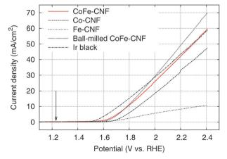
**Fig. 4** The OER activity of the CoFe-CNFs, Co-CNFs, Fe-CNFs, ball-milled CoFe-CNFs, and Ir black. The metal loading amount of the Me-CNFs and Ir black on GC is the same,  $40~\mu g~cm^{-2}$ . The arrow mark in this figure indicates the equilibrium potential of the ORR/OER.
