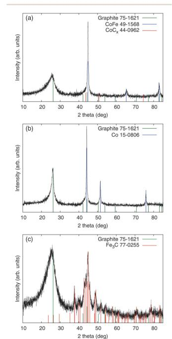
Fig. 2 XRD results of the (a) CoFe-CNFs, (b) Co-CNFs, and (c) Fe-CNFs.
