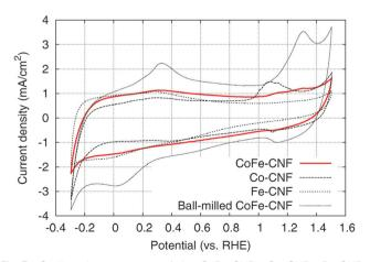
Fig. 3 Cyclic voltammograms of the CoFe-CNFs, Co-CNFs, Fe-CNFs, and ball-milled CoFe-CNFs in 0.1 M KOH aqueous solution at a scan rate of 50 mV s $^{-1}$ .
