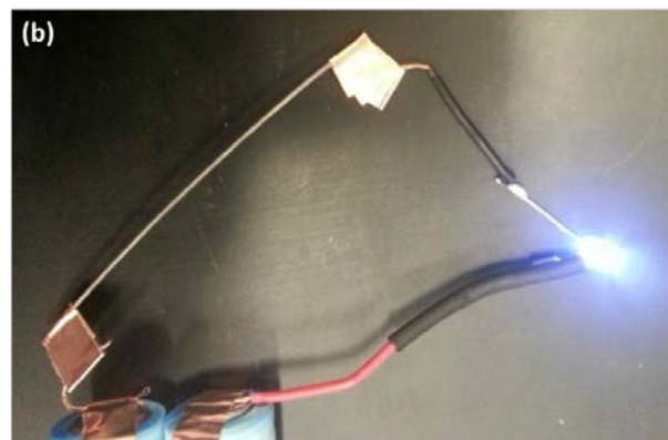
Fig. 3 (a) Current-voltage curves of nylon thread coated with different nanowire densities. (b) Passing current through nanowire-coated nylon thread (top left of image) to power an LED
