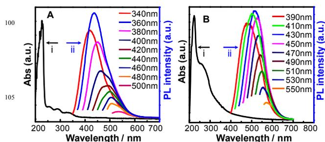
Figure 4. UV-vis absorption spectra (i) and photoluminescence spectra (ii) for the simultaneously prepared CDs. (A) hydrophilic CDs and (B) hydrophobic CDs.
