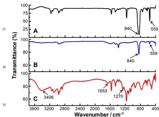
Figure 2. FT-IR spectra of the ionic liquid serving as carbon source and the simultaneously prepared CDs. (A) BmimPF<sub>6</sub>, (B) hydrophobic CDs, (C) hydrophilic CDs.
