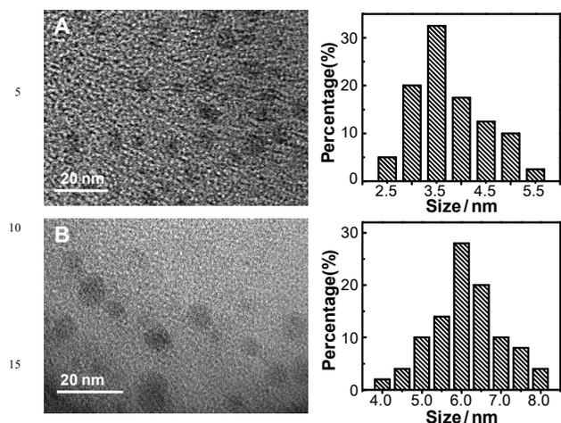
Figure 1. HRTEM images and size distribution histograms for the simultaneously prepared hydrophilic CDs (A) and hydrophobic CDs (B).
