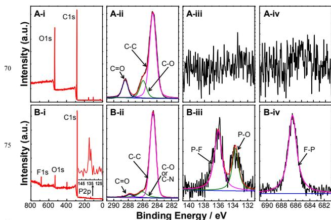
Figure 3. XPS spectra for the simultaneously prepared CDs. (A) hydrophilic CDs, (B) hydrophobic CDs. (i) raw data, (ii) high resolution spectra of C1s, (iii) P2p, (iv) F1s.
