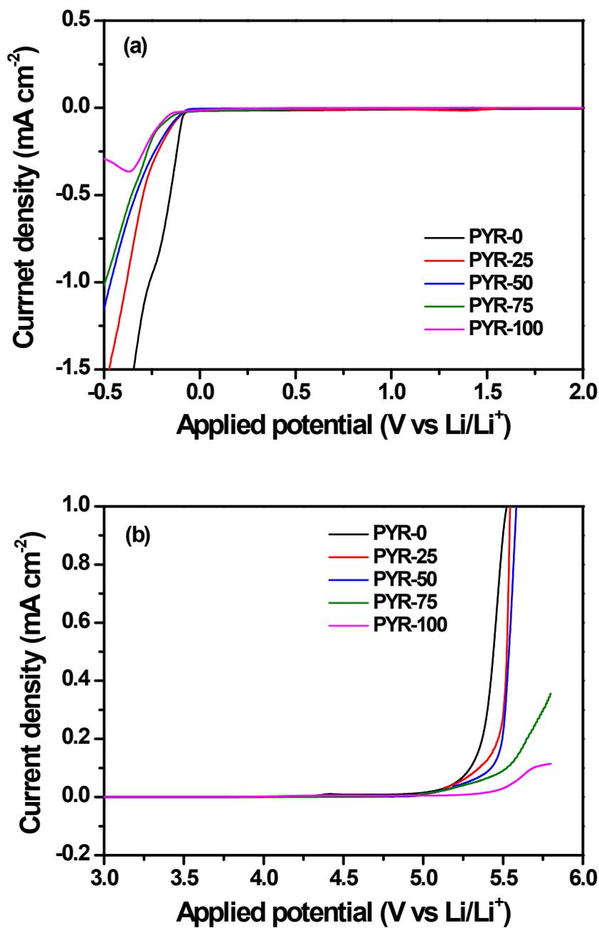
**Fig. 4.** Linear sweep voltammograms of the mixed electrolytes containing different contents of MEEsPyr-TFSI: (a) cathodic scan and (b) anodic scan (scan rate: 1 mV s<sup>-1</sup>, temperature: 25 °C).
