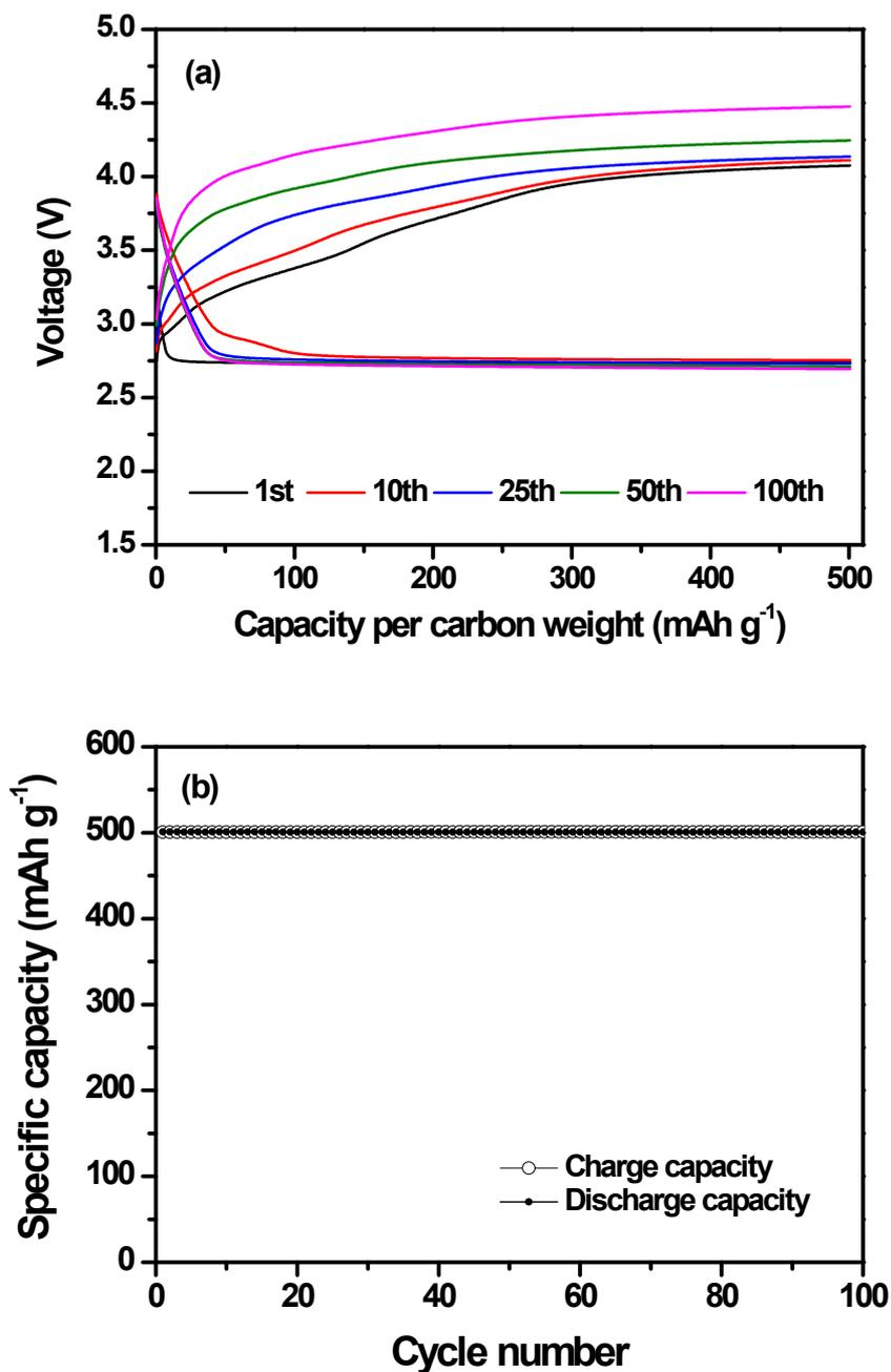
**Fig. 8.** (a) Discharge and charge curves of lithium-oxygen cells assembled with PYR-25 electrolyte at a constant current density of  $0.1 \text{ mA cm}^{-2}$  ( $100 \text{ mA g}^{-1}$ ); the capacity utilization was limited to  $500 \text{ mAh g}^{-1}$ . (b) Discharge and charge capacities as a function of the cycle number. Carbon loading in the carbon electrode was  $1.0 \text{ mg cm}^{-2}$ .
