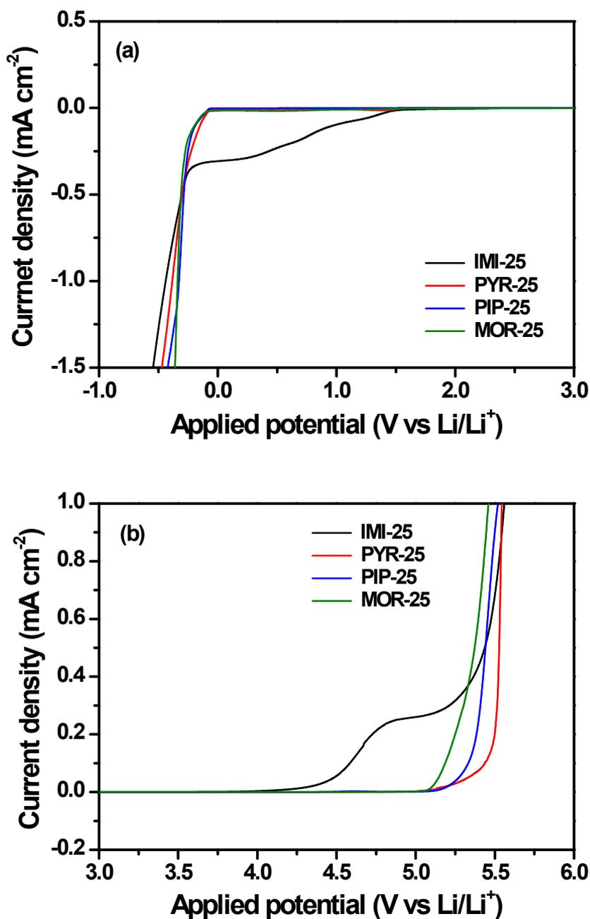
**Fig. 3.** Linear sweep voltammograms of the mixed electrolytes composed of 25 vol% ionic liquid and 75 vol% TEGDME: (a) cathodic scan and (b) anodic scan (scan rate: 1 mV s<sup>-1</sup>, temperature: 25 °C).
