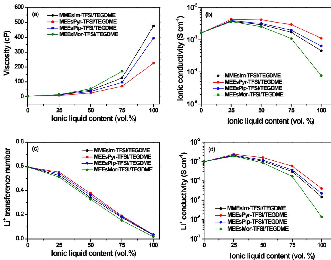
**Fig. 2.** (a) Viscosities, (b) ionic conductivities, (c) lithium transference number and (d) lithium ionic conductivities of the mixed electrolytes composed of different ionic liquids and TEGDME as a function of the ionic liquid content. MEEsMor-TFSI is solid at room temperature and thus, its viscosity could not be measured.
