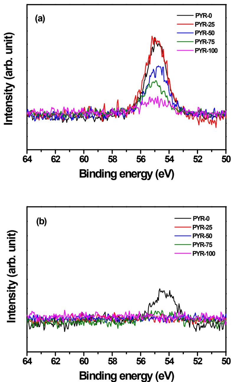
**Fig. 6.** Li 1s XPS spectra of the carbon electrodes employing different electrolytes (a) in the fully discharged state at 2.0 V and (b) in the fully charged state at 4.7 V.
