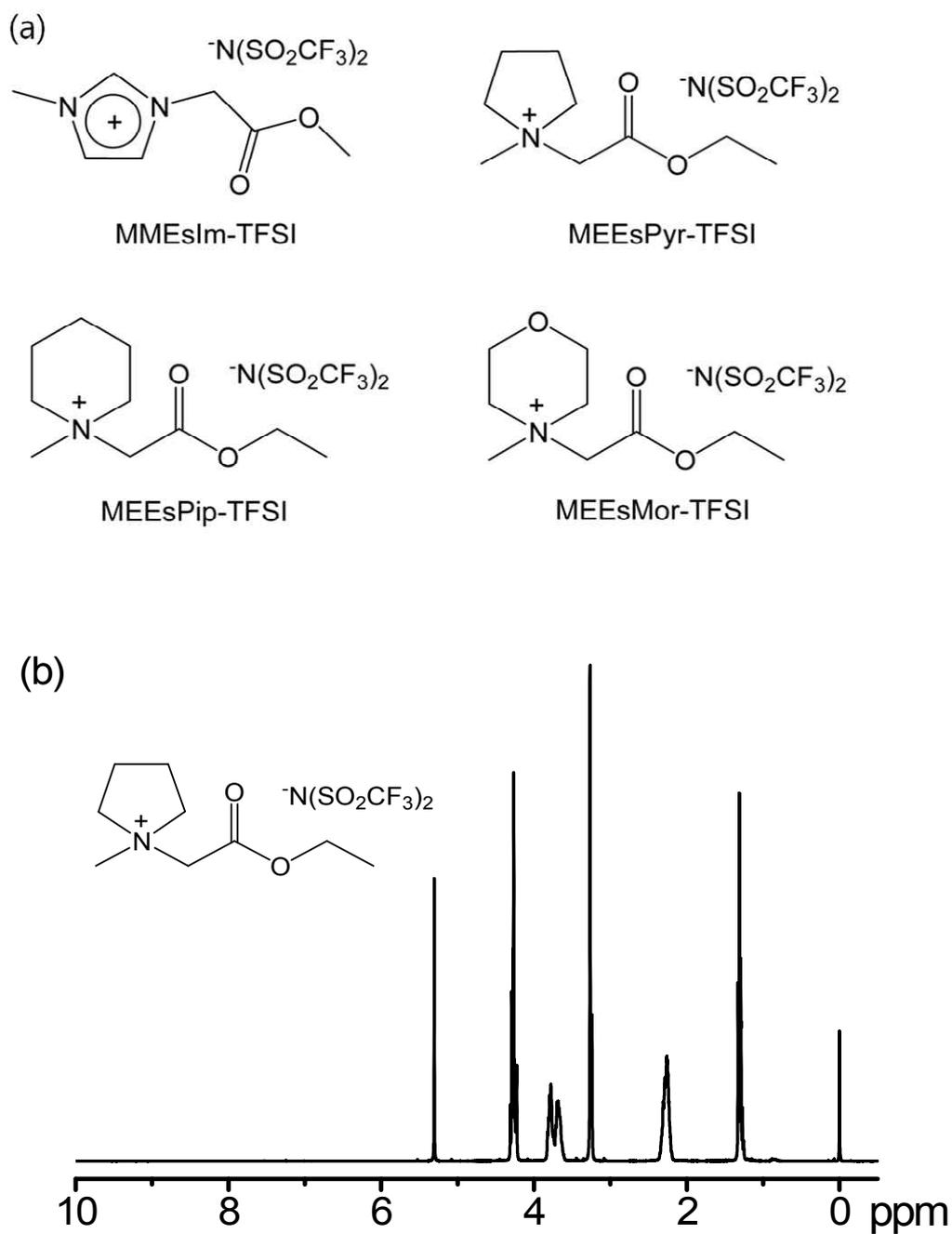
**Fig. 1.** (a) Chemical structures of the ionic liquids synthesized in this study and (b)  $^1\text{H}$  NMR spectrum of MEEsPyr-TFSI in acetone- $d_6$ .
