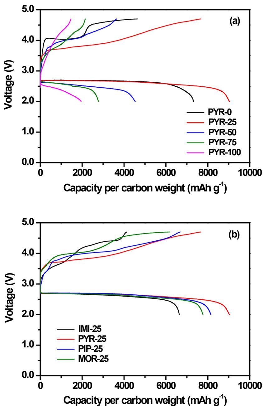
**Fig. 5.** Initial discharge and charge curves of lithium-oxygen cells assembled with (a) mixed electrolytes containing different contents of MEEsPyr-TFSI and (b) mixed electrolytes composed of 25 vol% ionic liquid and 75 vol% TEGDME. The cells were fully cycled between 2.0 to 4.7 V at a constant current density of  $0.1 \text{ mA cm}^{-2}$  ( $100 \text{ mA g}^{-1}$ ).
