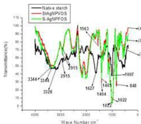
Fig.3. FTIR Spectra of Starch -Silver nano dichlorvos(a), nano-chlorpyrifos formulations (b) and Native starch (c)
