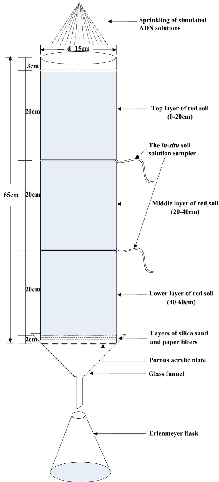
Fig. 1 Schematic sketch of the experimental setup.
