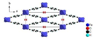
Figure 6. Structure of MIL-53(Fe) =  $Fe(OH/F)(BDC)\cdot[H_2O]$ , viewed along the c axis.
