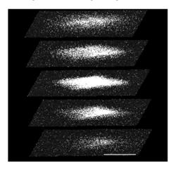
Figure 3: Sliced 3D image of a Fe(OH/F)(BDC)·[H<sub>2</sub>O] crystal displaying bulk Second Harmonic Generation. The scale bar on the bottom slice indicates a distance of 5  $\mu$ m. The interval between the slices is 6  $\mu$ m.
