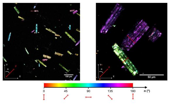
Figure 5. SHG polarization map. In the images each pixel is color coded, representing the angle (α) between the polarization and the Y-axis of the image. The polarization direction P is shown explicitly for two crystals on the right image (indicated by the red arrows).
