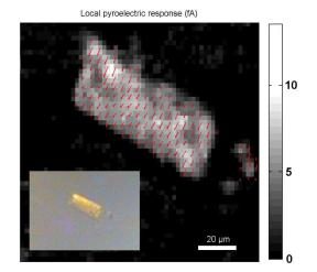
Figure 7: The local pyroelectric response map reveals a unipolar response from the Fe(OH/F)(BDC)-[H<sub>2</sub>O] crystal. Modulation frequency is 2025 Hz, laser power is 100 mW. Inset: Optical image.
