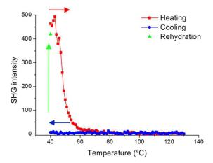
Figure 4. SHG signal of Fe(OH/F)(BDC)-[butanol] during a heating / cooling / rehydration cycle. The SHG signal vanishes completely during heating under N<sub>2</sub> flow and remains zero upon cooling. Heating and cooling occurred at 1°C/min under N<sub>2</sub> flow. In a last step, the SHG activity was recovered by allowing H<sub>2</sub>O molecules to enter the pores.
