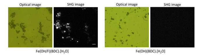
Figure 2. Optical and SHG images of MIL-53(Fe), synthesized in the presence or absence of fluoride. Fe(OH/F)(BDC)·[H<sub>2</sub>O] generates SHG, indicating the occurrence of a non-centrosymmetric ordering. The scale bar on the left SHG image indicates a length of 50 μm and is the same for all images.
