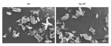
Figure 1. SEM images of MIL-53(Fe)[H<sub>2</sub>O] synthesized with (left) and without HF (right). The scale bar at the bottom right indicates a length of 20 µm.
