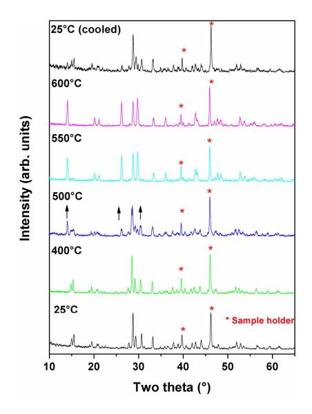
Fig. 3. Typical XRD patterns of  $K_2Ce(PO_4)_2$  recorded at different temperatures (( $\lambda = 1.5417\text{Å}$ ). The upward arrows indicate the evolving high temperature phase and asterisks indicate the peaks due to platinum sample holder. The XRD patterns at 550 and 600°C are representatives for the high temperature phase of  $K_2Ce(PO_4)_2$ .
