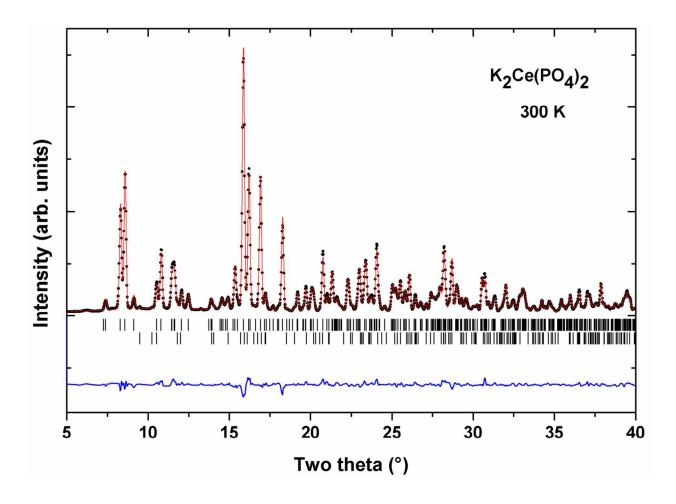
Fig. 4: Rietveld refinement plot of the powder XRD pattern of  $K_2Ce(PO_4)_2$  composition ( $\lambda = 0.8584 \text{ Å}$ ). Lower vertical ticks are the Bragg positions for monoclinic CePO<sub>4</sub>.
