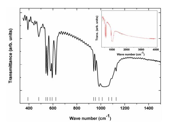
Fig. 10: Typical IR spectrum of K<sub>2</sub>Ce(PO<sub>4</sub>)<sub>2</sub>.
