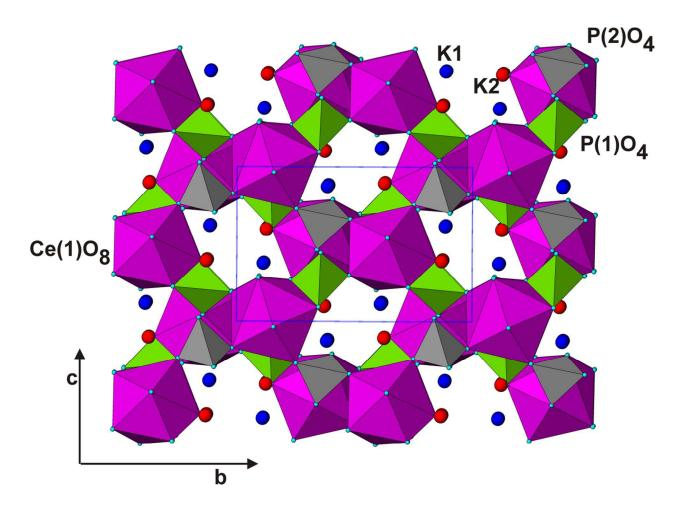
**Fig. 5:** Crystal structure of K<sub>2</sub>Ce(PO<sub>4</sub>)<sub>2</sub> in 100 projection. The CeO<sub>8</sub> (pink) and PO<sub>4</sub> tetrahedra (green and grey) are shown. Isolate spheres are K1 (blue) and K2 (red). Small (cyan) spheres indicate polyhedral corner oxygen atoms.
