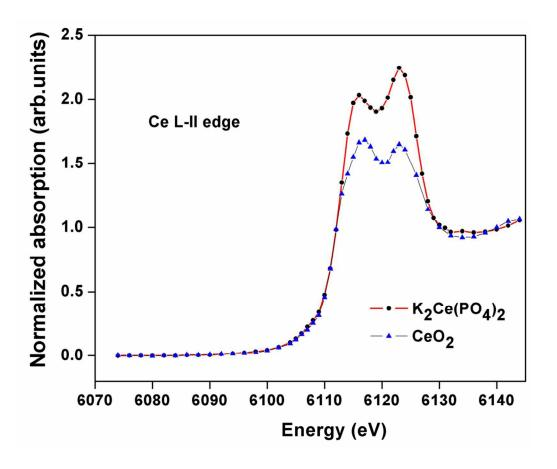
**Fig. 8:** XANES spectra of  $K_2Ce(PO_4)_2$  and  $CeO_2$  around the L-II edge.
