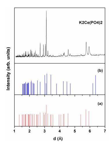
**Fig.1:** Powder XRD patters of different phases of  $K_2Ce(PO_4)_2$  composition ( $\lambda = 1.5417\text{Å}$ ). For comparison the data reported for  $K_4Ce_2P_4O_{15}$  (a) (ref 45) and  $K_2Ce(PO_4)$  H<sub>2</sub>O (b) (ref 43) are shown as vertical lines.
