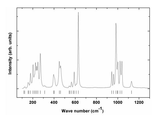
Fig. 9: Typical Raman spectrum of  $K_2Ce(PO_4)_2$ .
