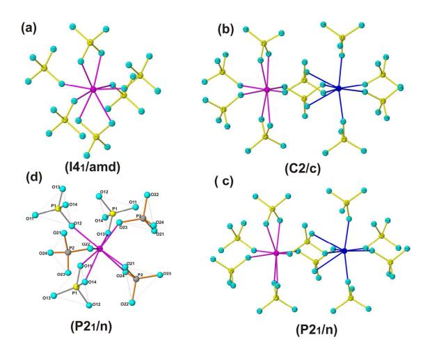
**Fig. 6:** Typical connections of distorted cubic  $MO_8$  polyhedra and tetrahedral  $PO_4$  in different  $A_2M(PO_4)_2$  structures.  $(NH_4)_2Ce(PO_4)_2H_2O$  (a.)  $ref\ 27,49$ ), (b) and (c) for  $Na_2Th(PO_4)_2(ref\ 57)$  and (d)  $K_2Ce(PO_4)_2$  of present study. Pink and blue spheres are  $M^{4+}$  cations. , Yellow and cyan spheres are  $P^{5+}$  and  $O^{2-}$  ions.
