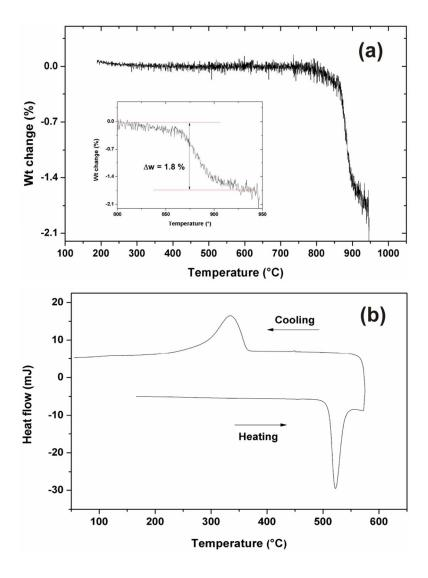
**Fig. 2:** Typical thermogravimetric curves of  $K_2Ce(PO_4)_2$  in heating cycle (a) and the DSC curves indicating the phase transition are shown in (b).
