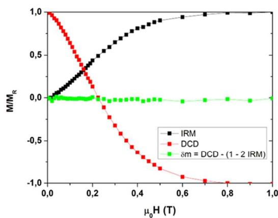
**Fig. 1.3:** IRM( $H$ ), DcD( $H$ ) and  $\delta m$  for annealed CoPt clusters embedded in an amorphous carbon matrix. The values presented here are divided by the remanent magnetization ( $M_R = IRM(\infty)$ ).
