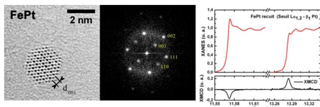
**Fig. 1.5:** Experimental HRTEM image and corresponding Fourier transform obtained on a FePt cluster where the chemical L1<sub>0</sub> order is visible (left). Evidence of induced magnetic moment in Pt from XMCD measurement at L<sub>2,3</sub> Pt edge (right).
