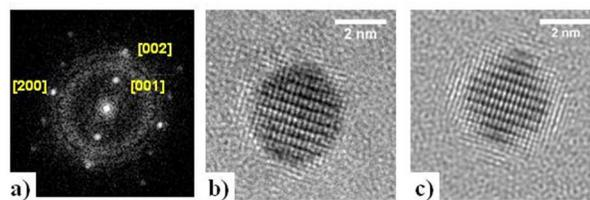
**Fig. 1.2:** a) Fourier transform of the experimental HRTEM image of a CoPt cluster where the chemical L1<sub>0</sub> order is visible. b) The [001] peak is the signature of the chemical order in the nanoparticle. c) Simulated HRTEM image of a perfectly ordered cluster.
