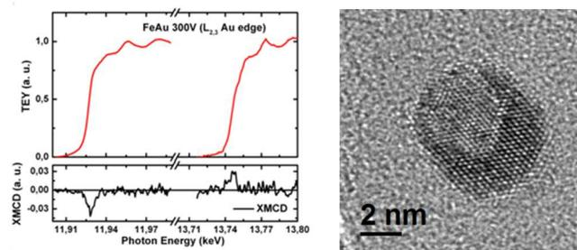
**Figure 3.1:** Evidence of induced magnetic moment on Au atoms from XMCD measurement at the  $L_{2,3}$  Au edge (left) for as-prepared FeAu clusters (around 3 nm diameter) embedded in amorphous carbon. HRTEM image of an annealed CoAu nanoparticle (capped with carbon), displaying a core/shell structure with an off-centered Co core surrounded by an Au shell.
