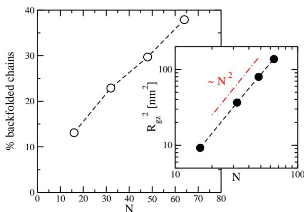
**Fig. 2** Main panel: Percentage of chains in a melt having at least one hairpin, as a function of number of chain segments,  $N$ . Inset: The component of the average radius of gyration (squared),  $R_{gz}^2$ , along the director as a function of  $N$ .
