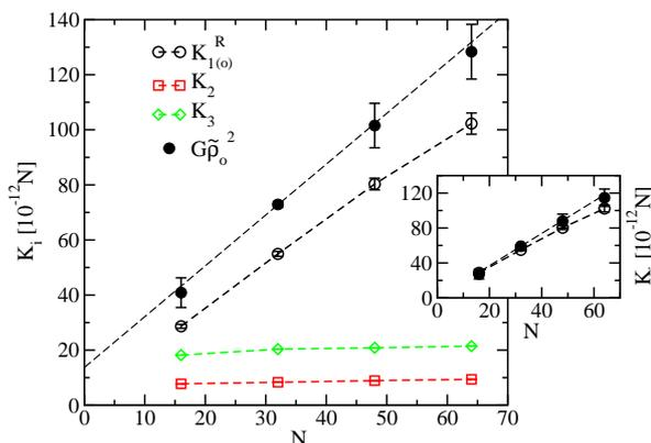
**Fig. 7** Main panel: Splay,  $K_{1(o)}^R$ , twist,  $K_2$ , and bend,  $K_3$ , elastic constants as a function of the number of segments in a chain. The  $G\tilde{\rho}_0^2$  calculated in Fig. 5 is also reproduced on the plot. Inset: Comparison of  $K_{1(o)}^R$  and  $G\tilde{\rho}_0^2$  after subtracting from the latter the offset indicated in Fig. 5.
