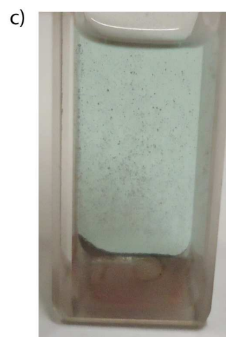
Figure 1. UV- vis spectra (a) and visual observation (b and c) of disproportionation of Cu(I)Br in TFE in the presence of various amounts of acetic acid recorded after 60 min of mixing reagents at 25 °C. Conditions: [Cu(I)Br] 0 = 16.5 mM, TFE = 1.8 mL, [Cu(I)Br] 0 /[Me 6 -TREN] 0 = 1/1.
