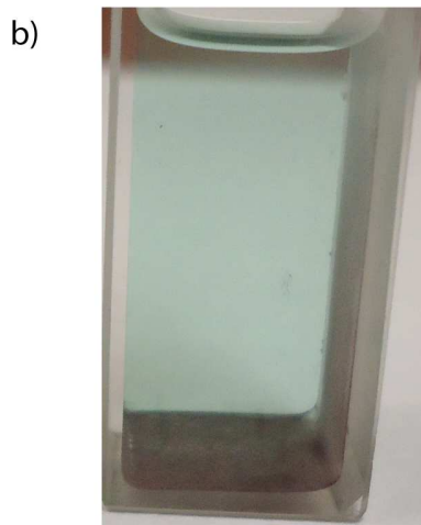
Figure 1. UV- vis spectra (a) and visual observation (b and c) of disproportionation of Cu(I)Br in TFE in the presence of various amounts of acetic acid recorded after 60 min of mixing reagents at 25 °C. Conditions: [Cu(I)Br] 0 = 16.5 mM, TFE = 1.8 mL, [Cu(I)Br] 0 /[Me 6 -TREN] 0 = 1/1.
